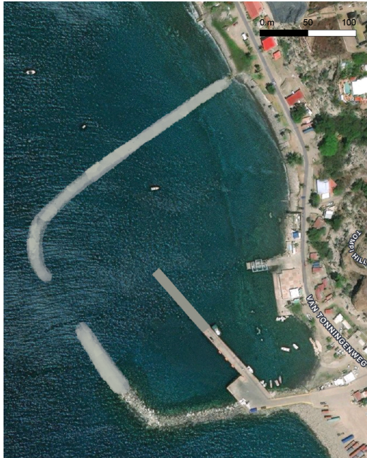
Figure 5.2: Breakwater design Harterink (2023)
