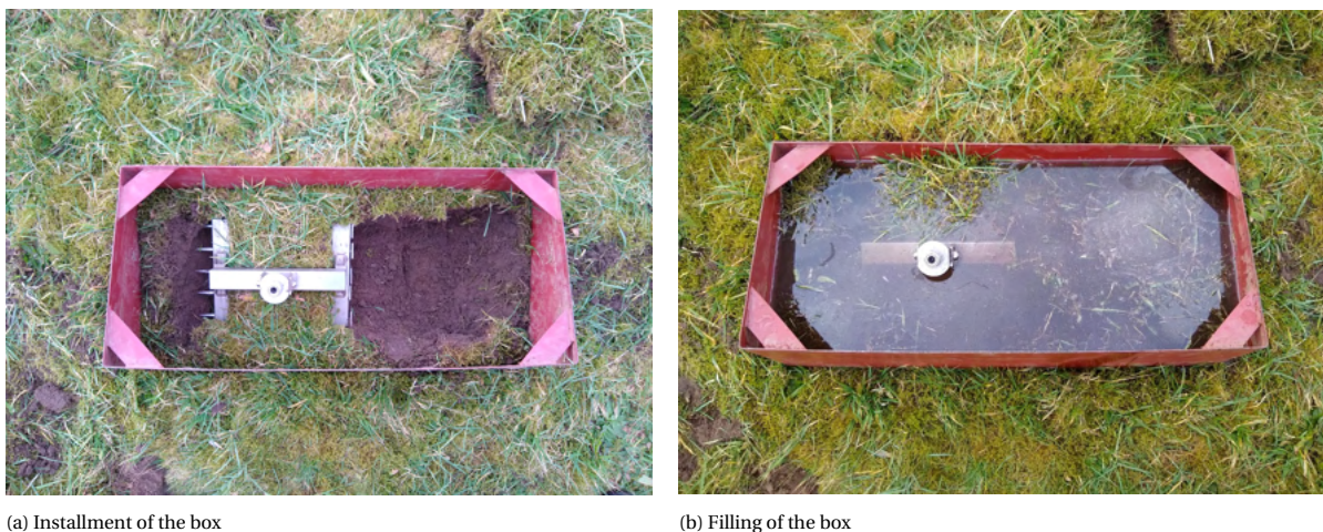
Figure 3.4: Installment and filling of the box for a submerged test
