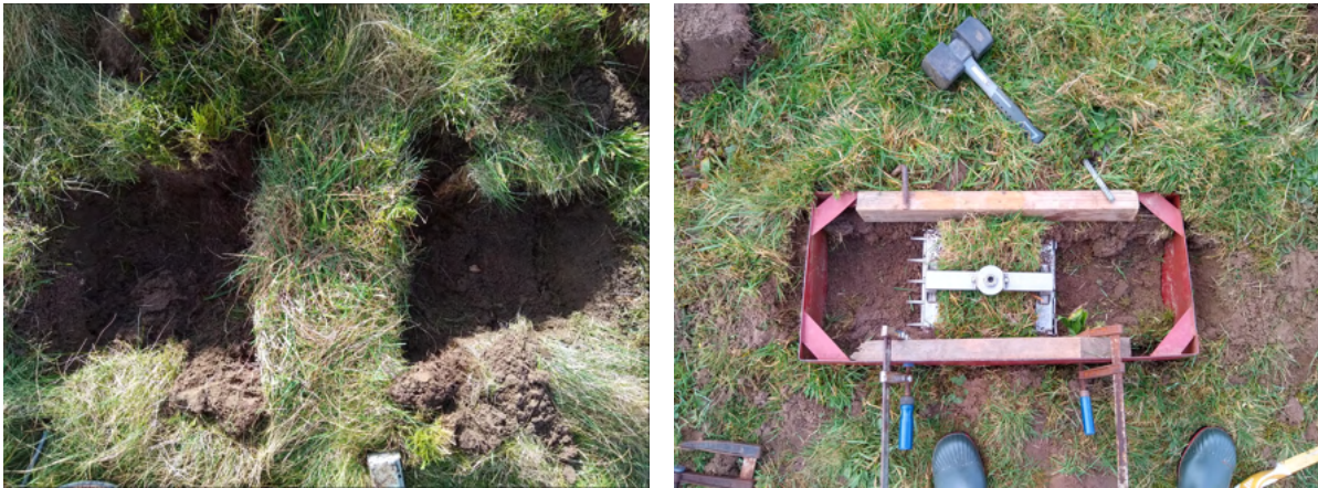
(a) Excavation for the shear test
