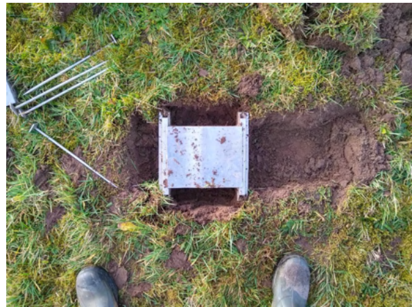
(b) Excavation around test sample
