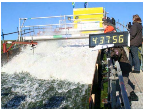
(a) Wave overtopping simulator. Adapted from: Van der Meer et al. (2009b)
