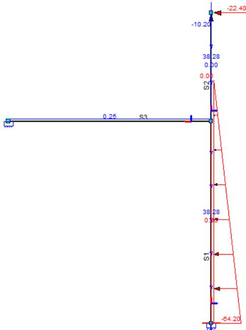
Figure 160 - Load case empty stilling basin full wave impact
