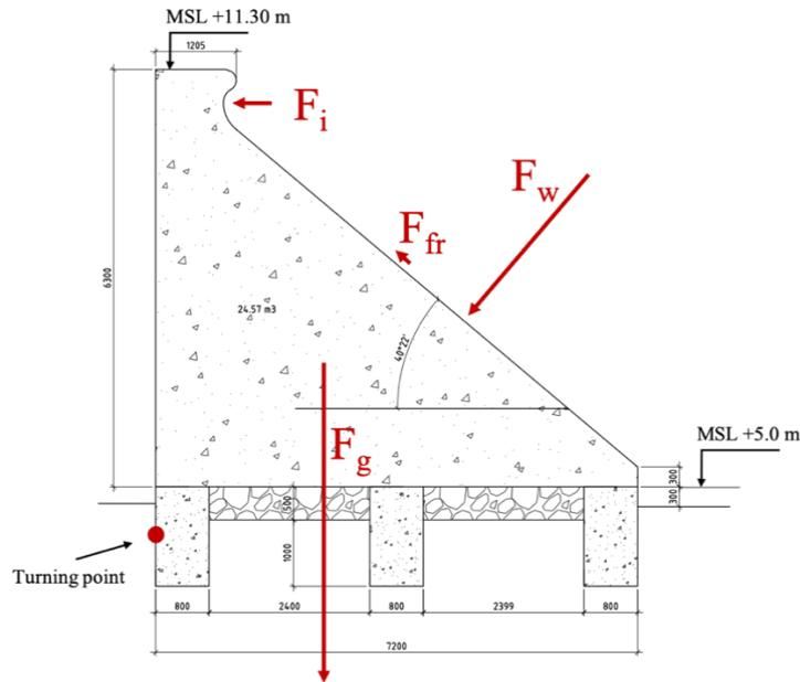
Figure 128 - Cross section of coastal defense part A in which the relevant forces for a stability analysis are displayed
