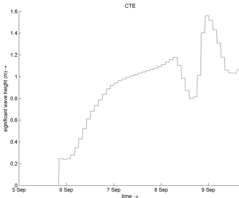
Figure 79 - Significant wave height at CTE, combination 1, large time step
