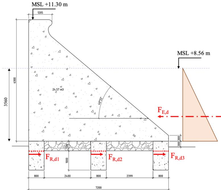
Figure 131 – Forces that could lead to internal instabilities
