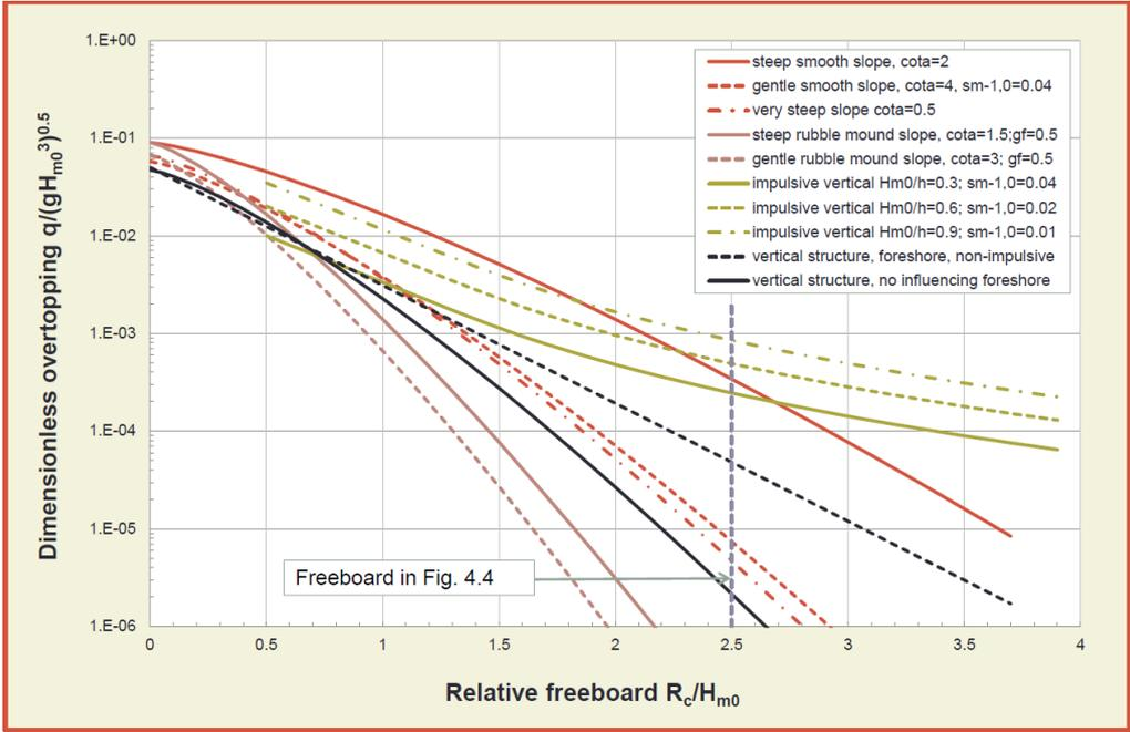
Figure 132 – Comparison of wave overtopping formulae for various kind of structures (EurOtop, 2018)
