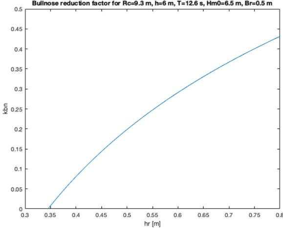
Figure 112 – A plotted bullnose reduction factor versus the height of the bullnose for a relatively large crest freeboard situation.
