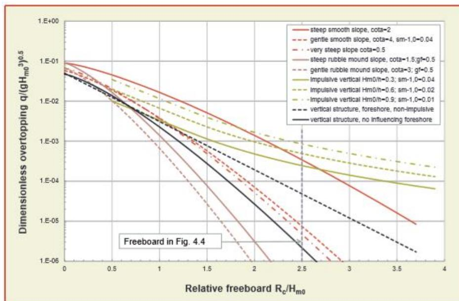
Figure 7 – Comparison of wave overtopping formulae for various kind of structures (Allsop N. W., et al., 2018)
