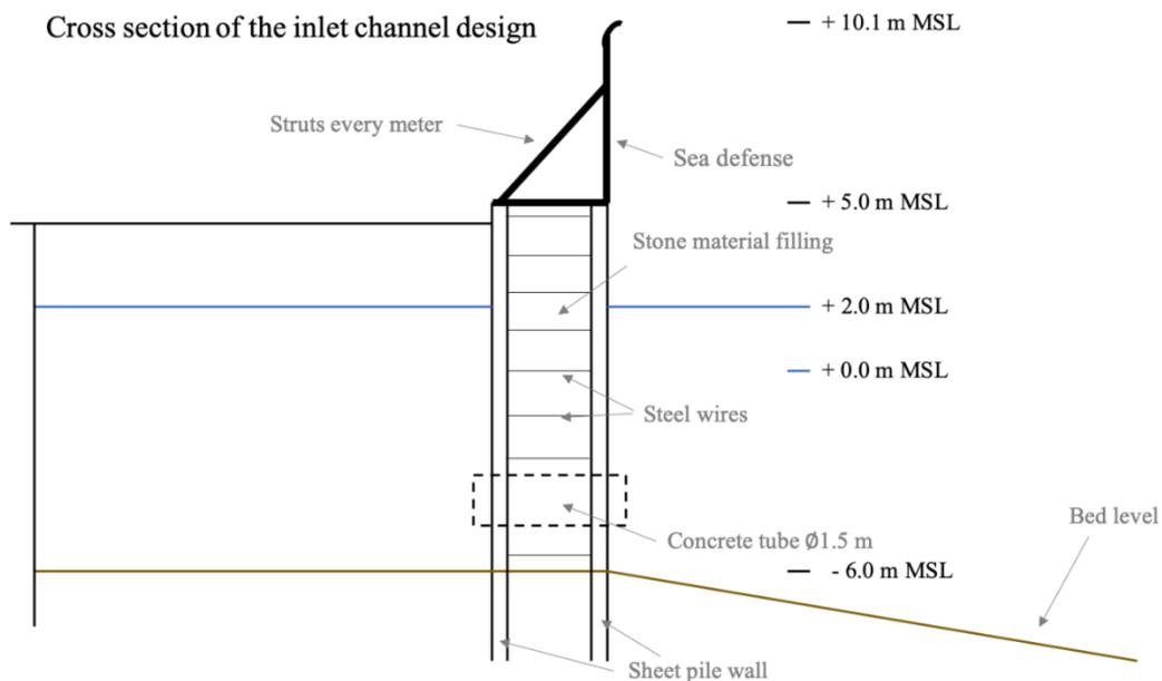
Figure 176 – Schematic cross section of the inlet channel with explanatory notes
