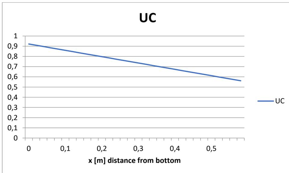
Figure 170 - Unity check vs distance from bottom, h = 250 mm
