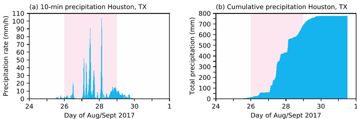
Figure 32 – 10-min precipitation rates and cumulative precipitation fallen in Houston, TX due to hurricane Harvey (van Oldenborgh, et al., 2017)
