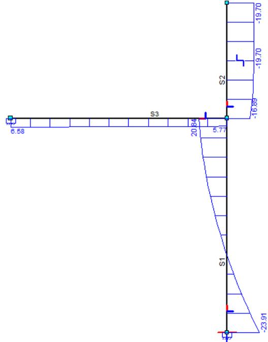
Figure 235 - Shear force diagram  $h = 4$  m
