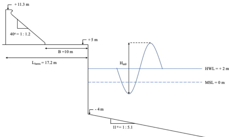
Figure 109 - Schematization current design section A-1
