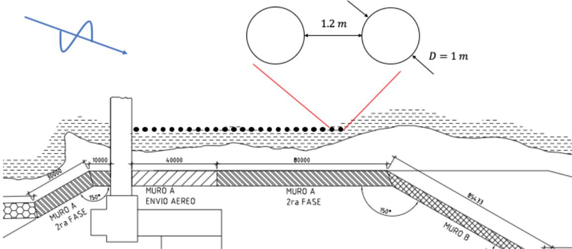
Figure 134 - Section A-1 pilescreen lay out
