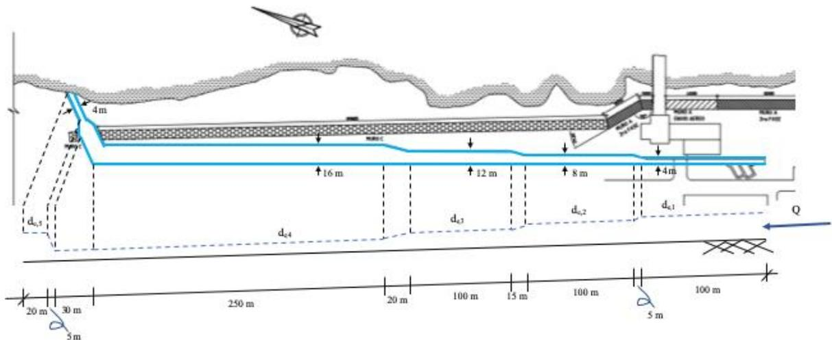
Figure 123 – Drainage channel under normal conditions
