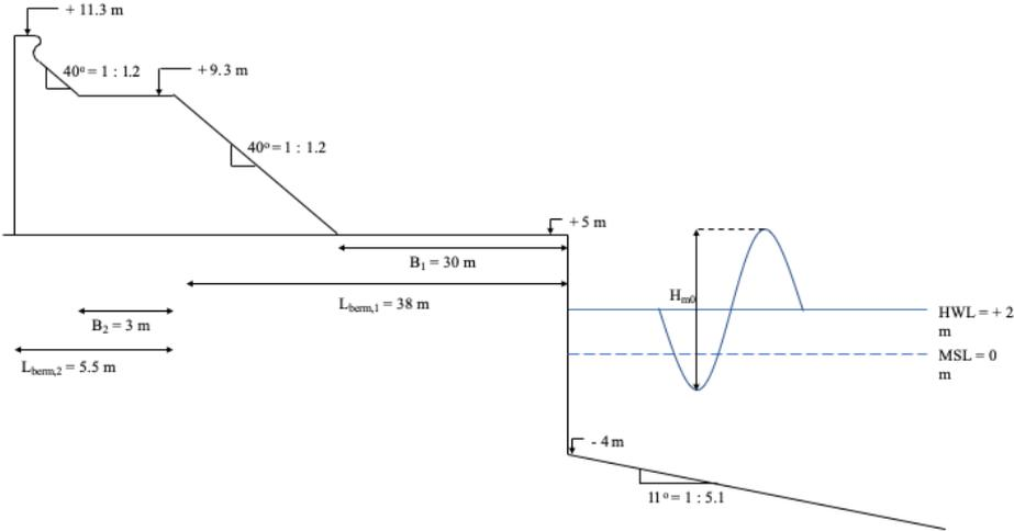
Figure 117 - Schematization section C
