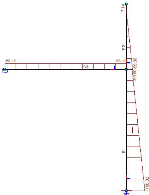
Figure 239 - Normal force diagram,  $h = 3$  m, wave impact
