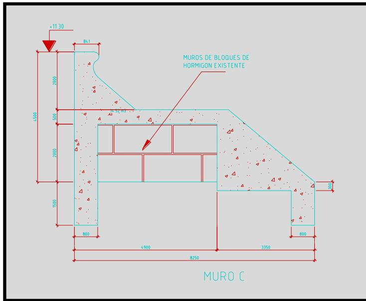
Figure 185 – Technical drawing of the current defense wall part C
