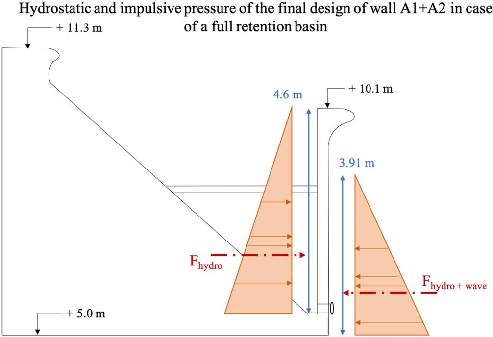
Figure 154 - Schematization hydrostatic pressures
