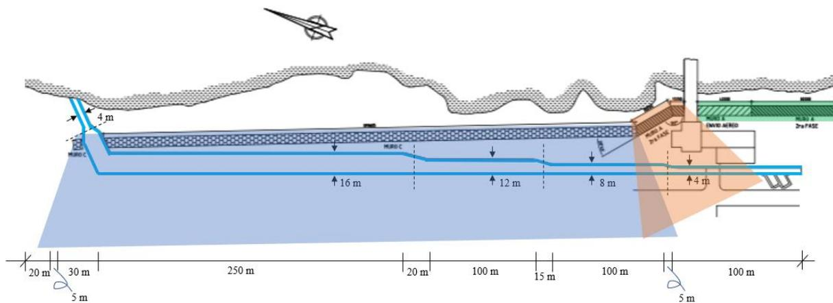
Figure 137 – Distribution of the overtopping. The blue area represents an overtopping of 45 l/s/m. The orange area represents an overtopping of 110 l/s/m.
