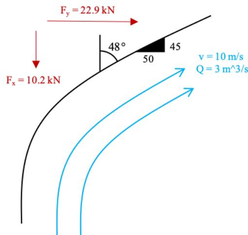
Figure 157 – Schematization of the forces on the bullnose due to the splashing water
