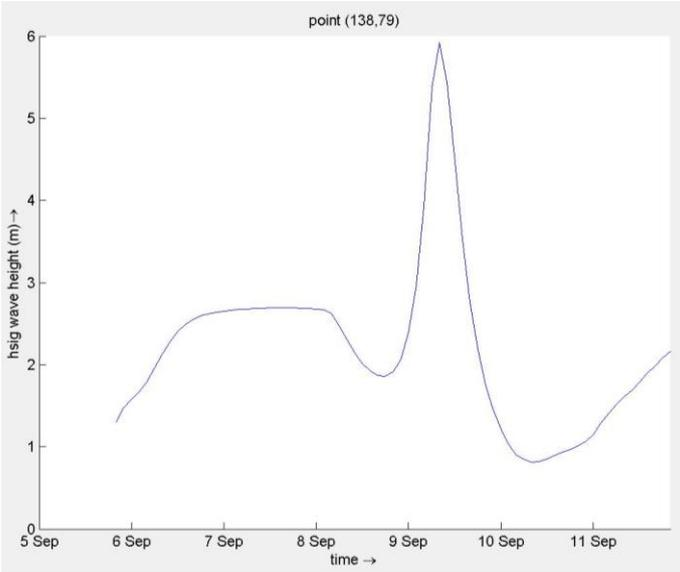
Figure 71 - Significant wave height Cayo Coco
