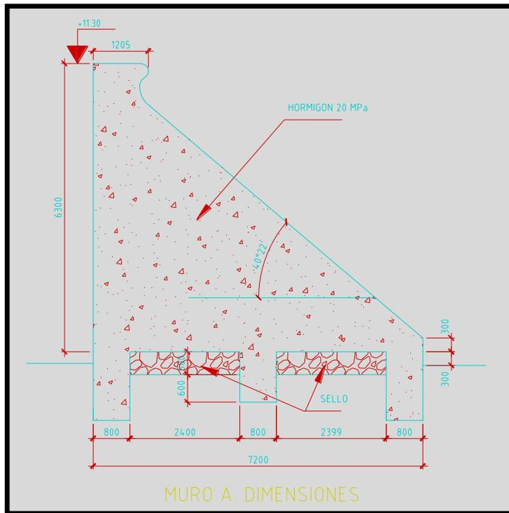
Figure 183 – Technical drawing of the current defense wall part A
