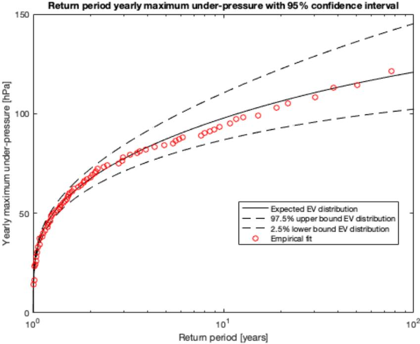
Figure 34 – GEV fit under-pressures
