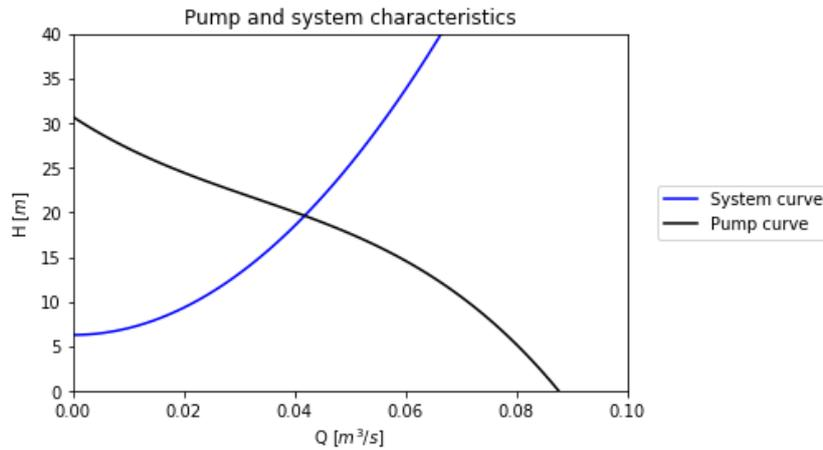
Figure 143 – Pump and system curves
