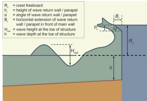
Figure 111 – Schematic figure of the parameters that determine the bullnose effectiveness.
