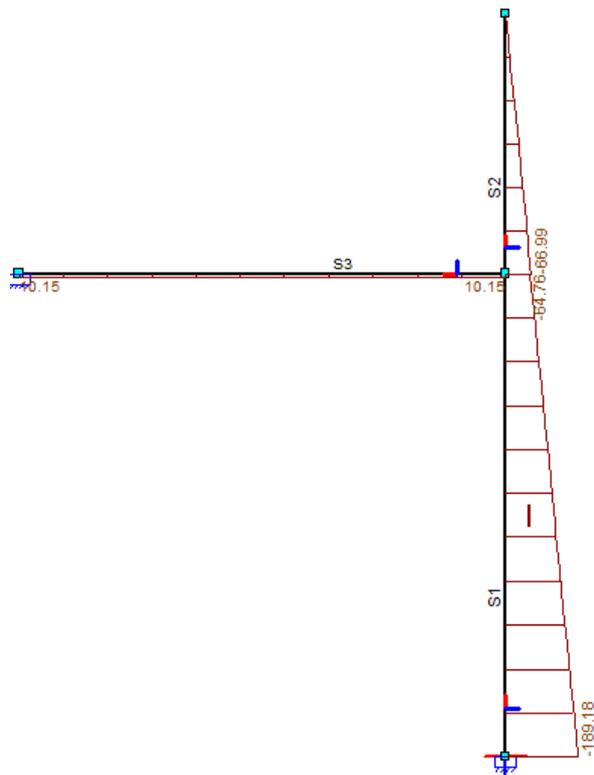
Figure 242 - Normal force diagram,  $h = 3$  m, no wave
