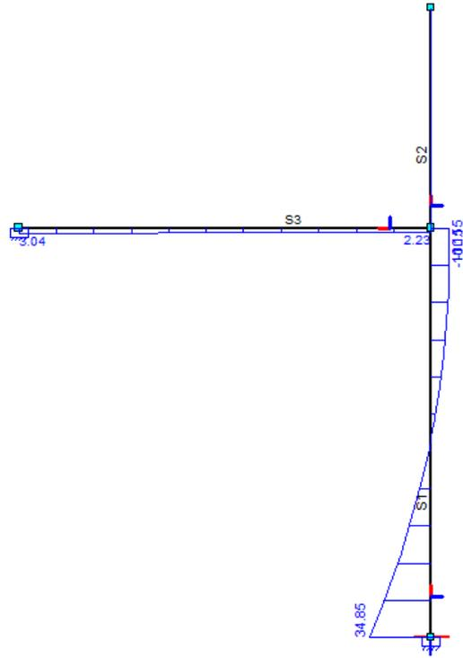
Figure 241 - Shear force,  $h = 3$  m, no wave
