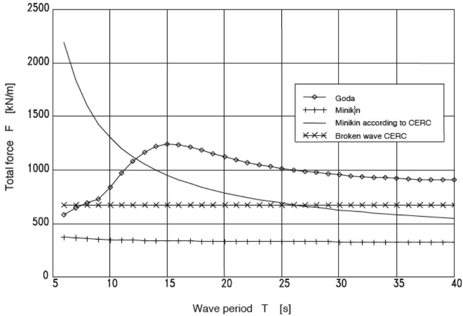
Figure 152- Comparison methods impulsive wave forces (TU Delft, 2019)
