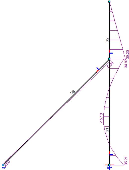
Figure 243 - Moment distribution wall inlet channel, only wave impact
