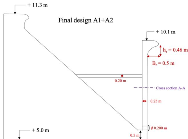
Figure 150 - Final design cross section A-1, A-2
