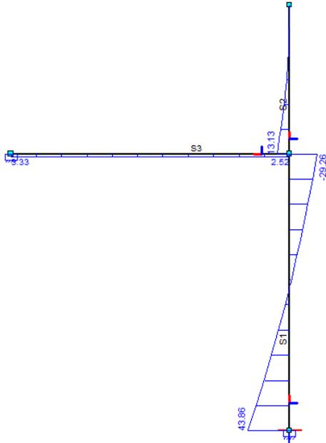
Figure 225 - shear force full basin no wave
