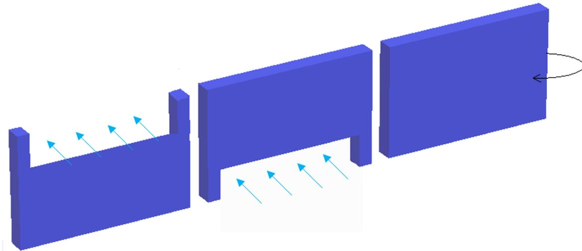
Figure 149 – The three types of gates, from left to right: submerged gate, culvert gate, regular gate
