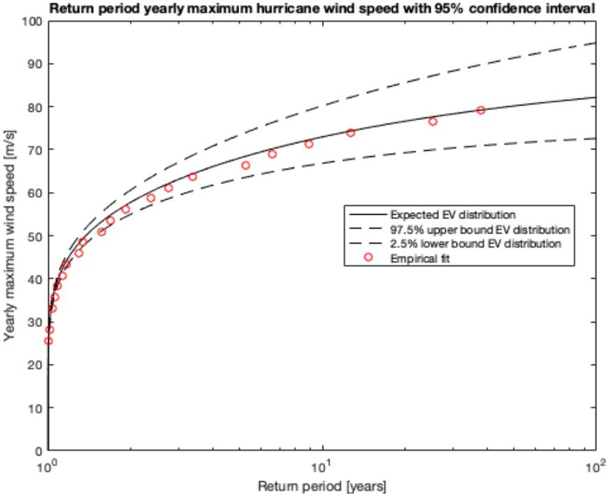
Figure 35 – GEV fit wind speeds
