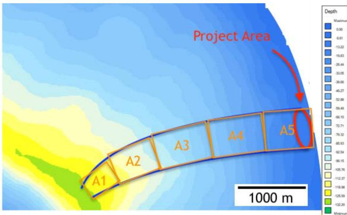
Figure 28 – Basic lay-out of run-off model (Deltares, 2019)
