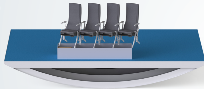
Figure 19. Concept 2: hand luggage space underneath the seat
