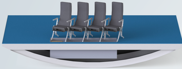
Figure 18. Concept 1: hand luggage space underneath the floor
