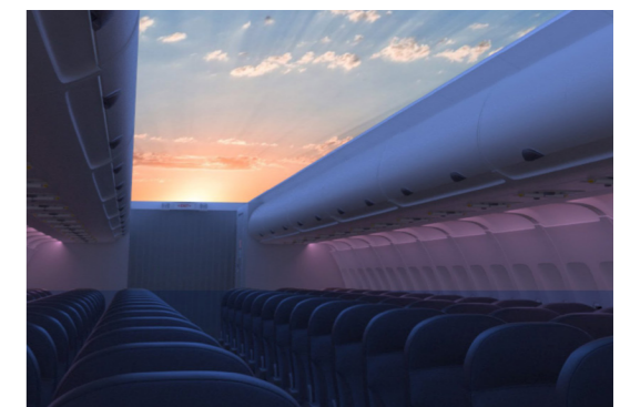
Figure 41. Light projections on the ceiling and overhead bins
