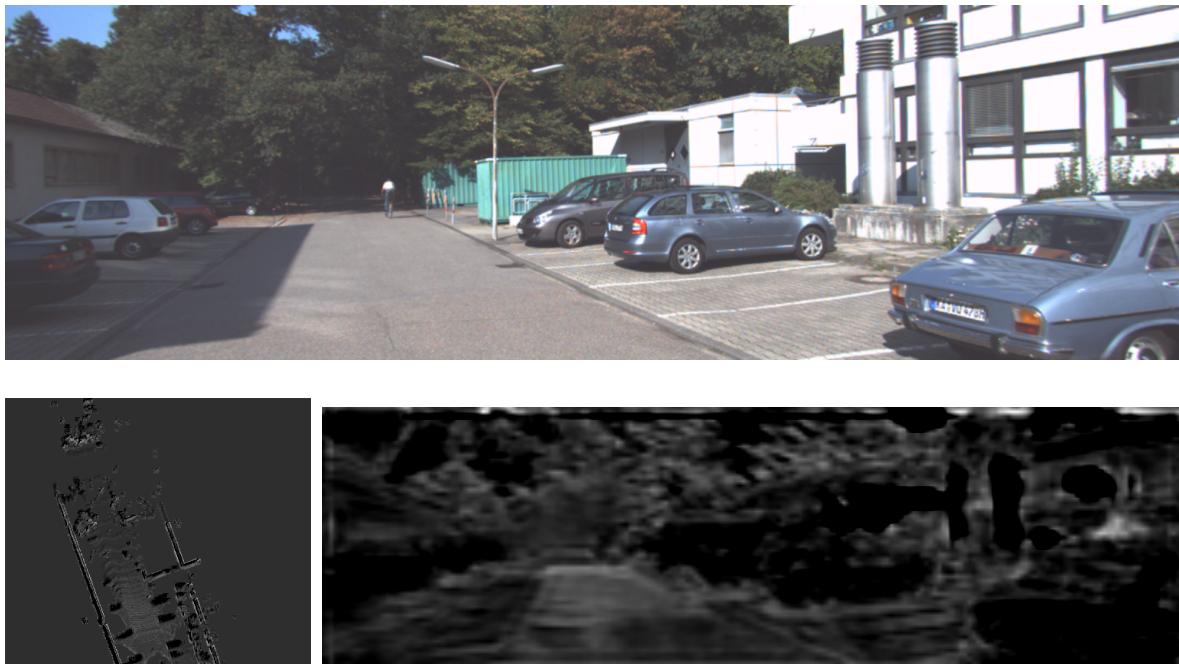
Figure 4-6: An example input image (top) and a corresponding point cloud feature map (bottom left) after 1 \times 1 convolution and an image feature map (bottom right). The feature are maps obtained in the training process.
