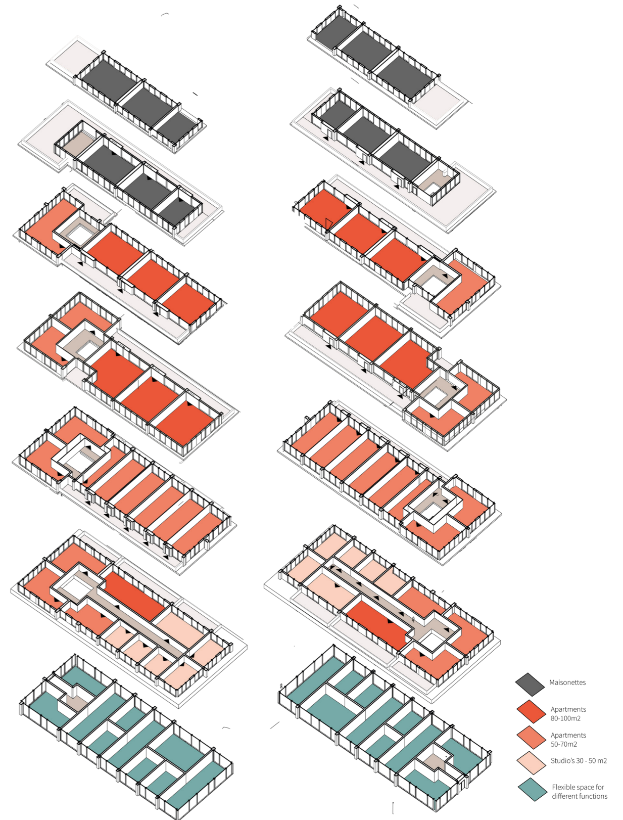
Figure 7.3. Different types of typologies within the block, in every layer the orientation is different
