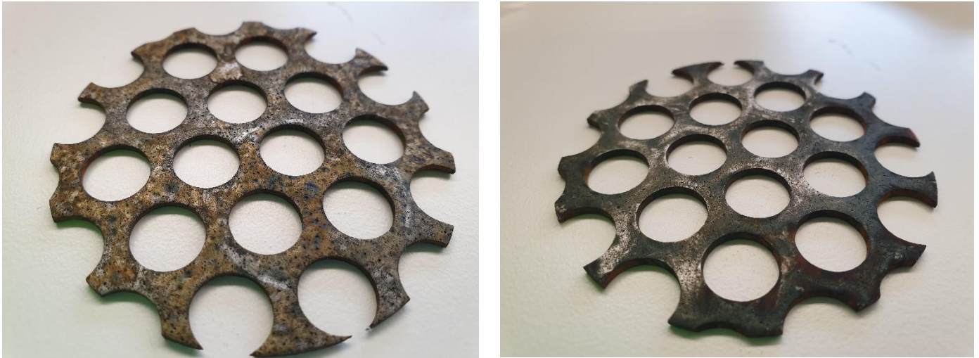
Fig. 23: Anode condition after 7 hours of operation for integrated electrodes in the reference experiments. Top of the horizontally placed anode (left) and bottom (right) with clear differences in surface layer formation
