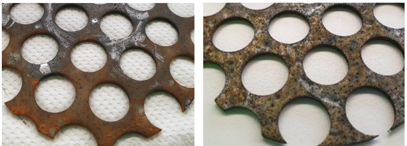
Fig. 26: Comparison of anode condition after operation when placed in the supernatant (left) and in the filter bed (right).
