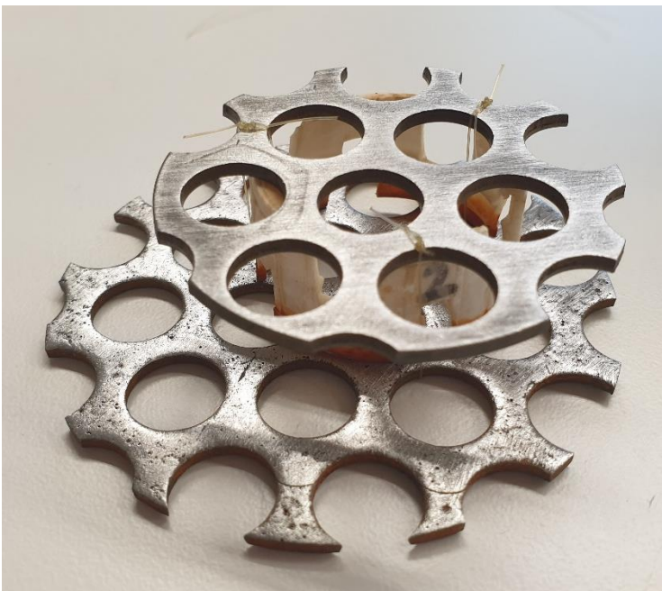
Fig. S1: Anode and cathode configuration (left) and connection of the electrodes to the DC power source (right). In this configuration the cathode anode can be seen on top of the anode, connected by nylon wire and a plastic spacer in between.
