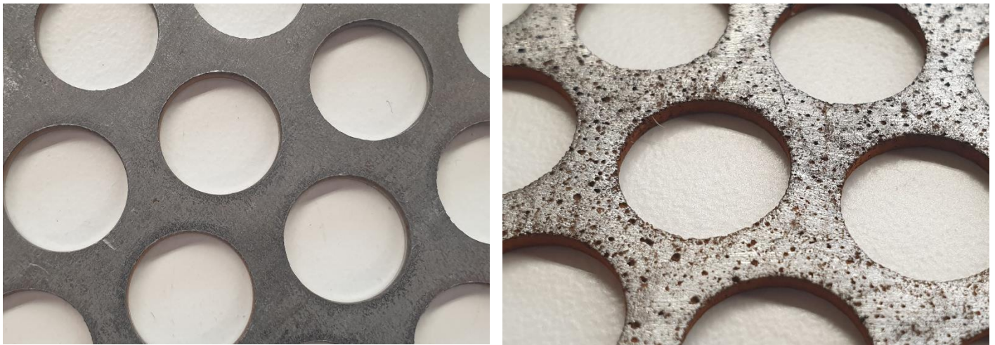
Fig. 27: Comparison of the surface on the top of the anode for the integrated electrodes. New anode (left) and previously used anode (right) with clear differences in smoothness of the surface caused by pitting corrosion.
