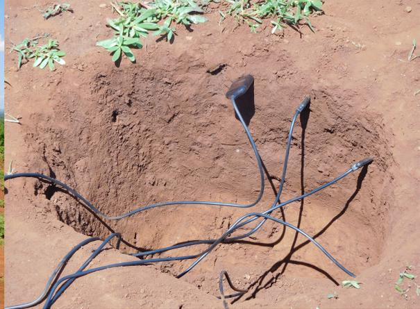
Figure 4.2: 5TM and EC5 sensors installed at the soil surface.
