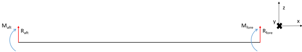
Figure 3.13: Shear force adjustment of the vessel section. Free body diagram with two equal oriented moments, M_{aft} and M_{fore} , applied on each end and the reaction forces, R_{aft} and R_{fore} , defined in positive z .
