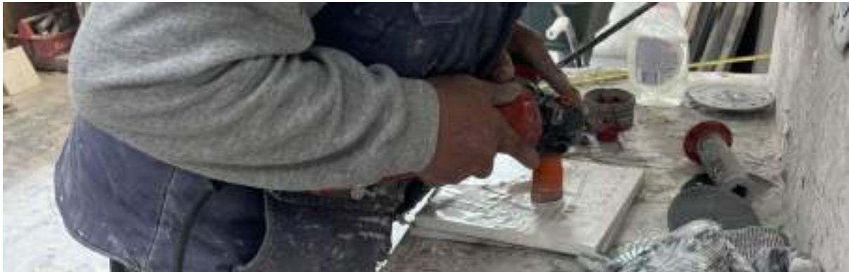
Fig X: The Lapitec sample being milled by hand with diamond headed drill.
