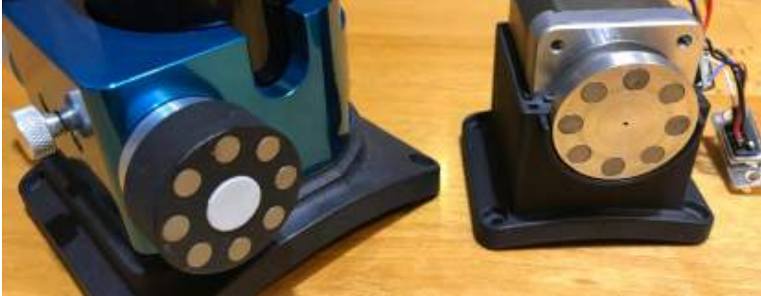
Fig x: Magnetic coupling posted by Markse68 on the Stargazers Lounge forum.
