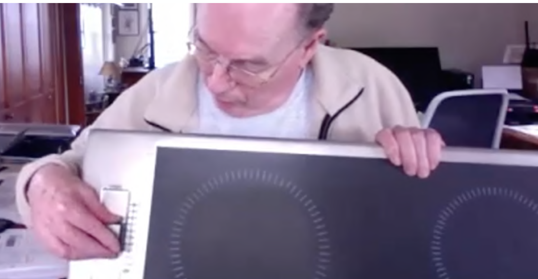
Fig 16: Terry showing the magnetic control knob of the Cool Top 2.
