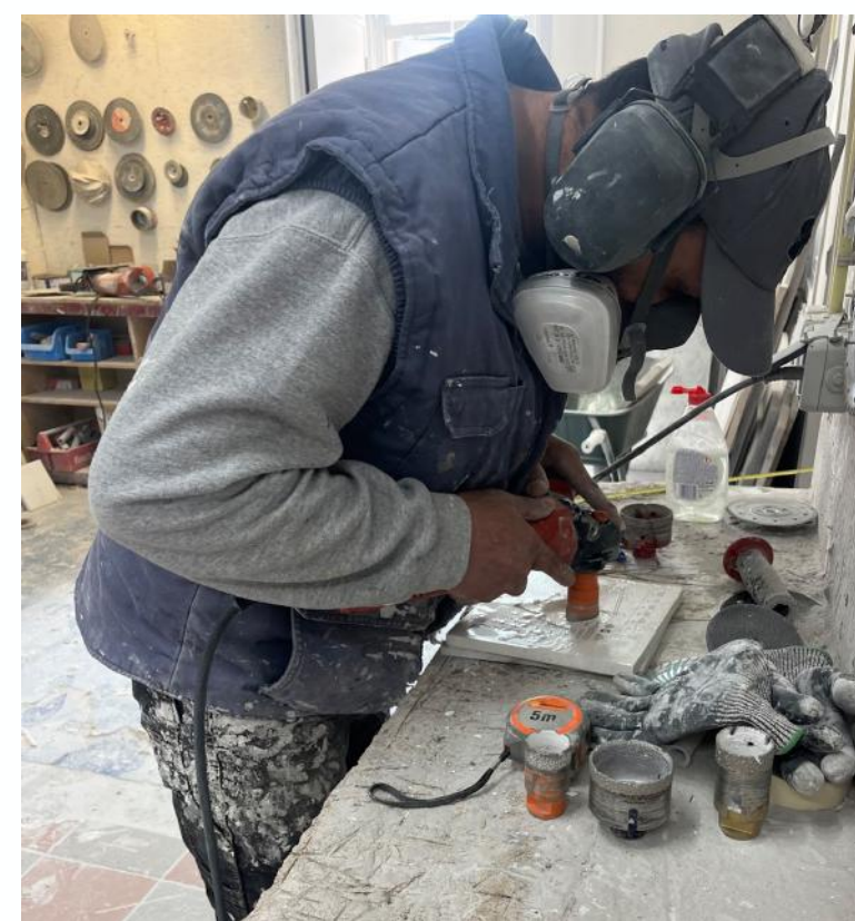
Fig 32: The Lapitec sample being milled by hand with diamond headed drill.
