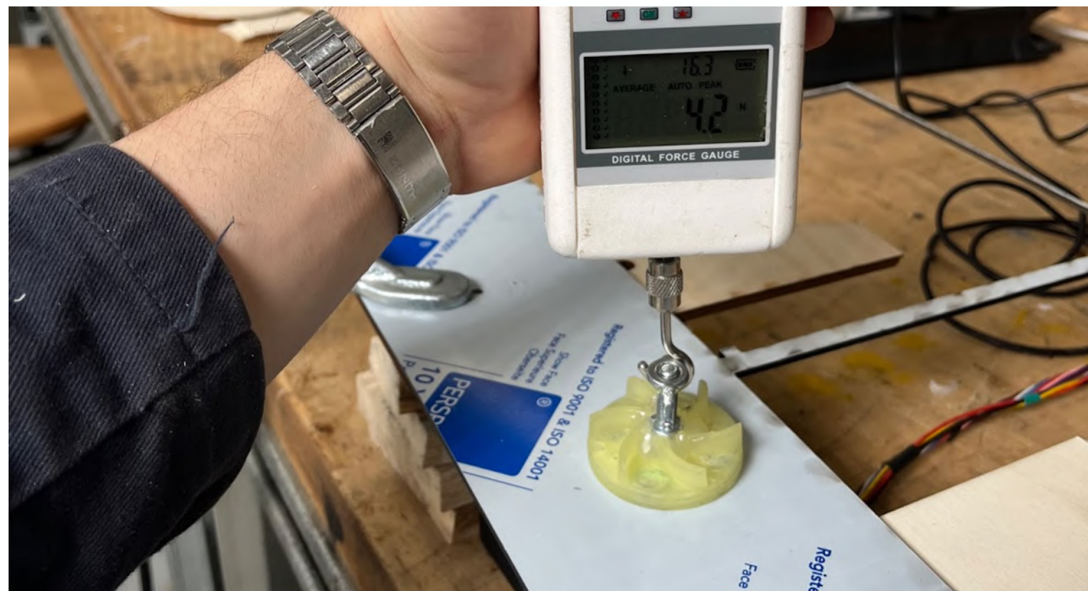
Fig 52: Measuring perpendicular disconnect force with a digital newton meter.
