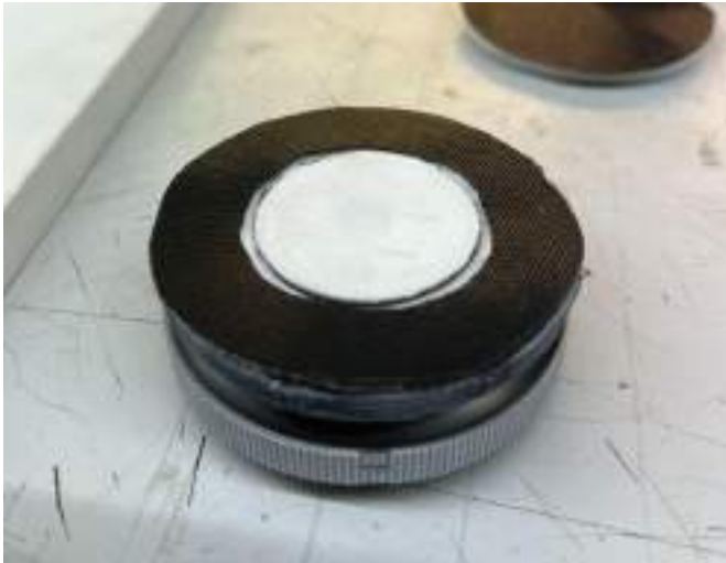
Fig X: PTFE pad cut to match the surface that was experiencing friction.
