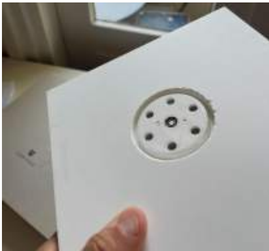
Fig x: Bottom coupling mounted on sample. Fig x: Top coupling mounted on sample.
