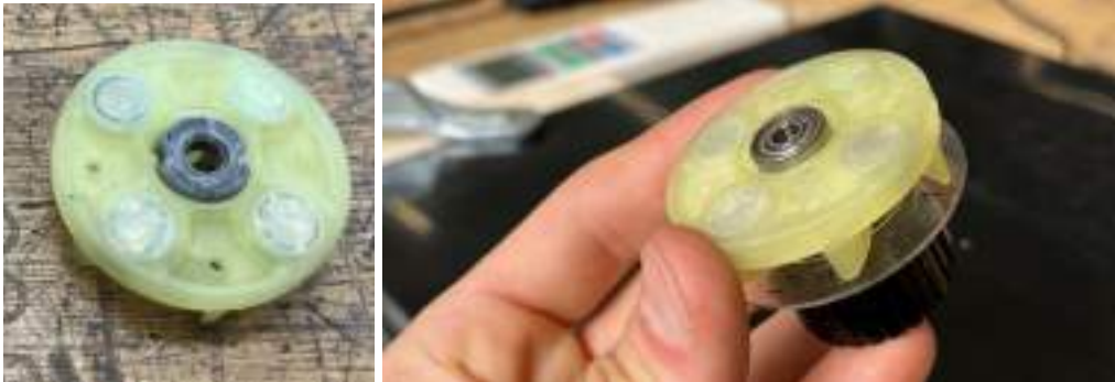
Fig x & x: Showing the magnetic coupling from the water pump with teflon and bearing respectively.
