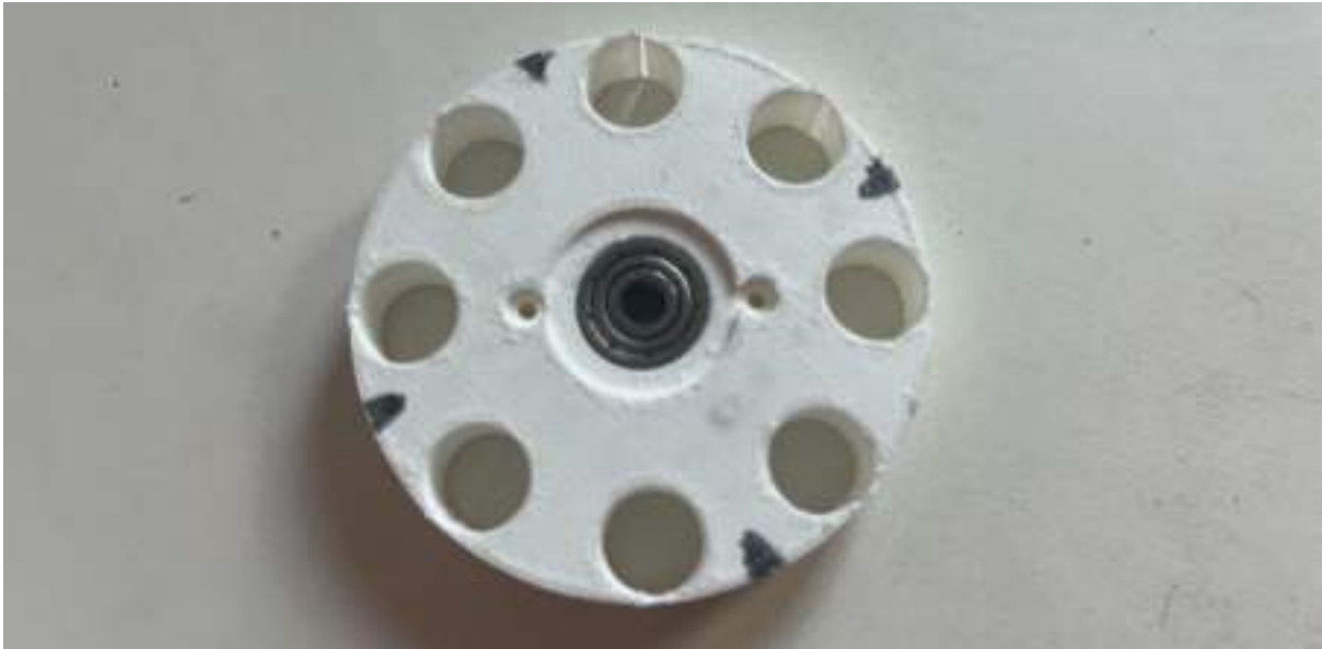
Fig x: The body shows room for coupling teeth between the magnets with pencil marks.
