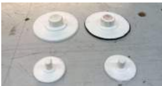
Fig: 3D printed bearing holder, 0.8mm gap left and 0.4mm gap
