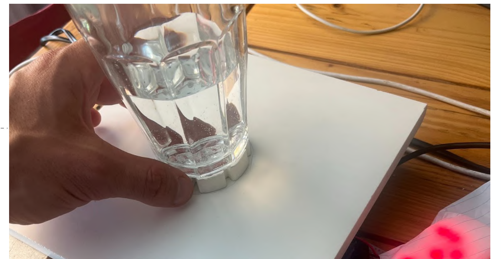
Fig 49: Fully 3D printed prototype with a glass of water in order to test a high weight scenario.
