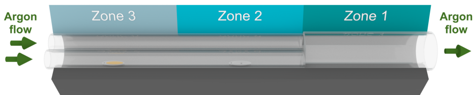
Figure 2.6: Schematic illustration of the three-zone gradient tube furnace from Carbolite Gero. This furnace is connected to an argon gas source at the entrance (at zone 3), and a bubbler system and subsequent exhaust at the back end (at zone 1). For the synthesis of WS 2 , sulfur powder is provided as chalcogen precursor in zone 3, while the substrate and tungsten-based precursor are loaded in zone 2.
