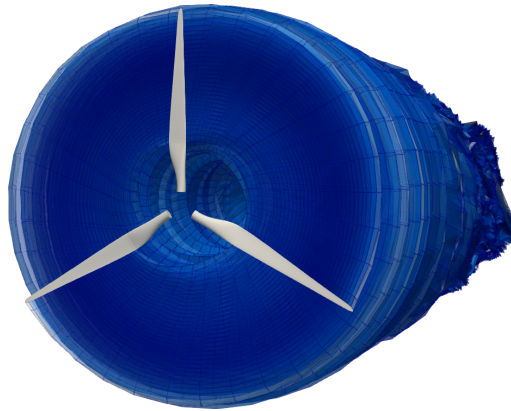
Figure 6. Panel method simulation results of the UNAFLOW rotor and its wake.
