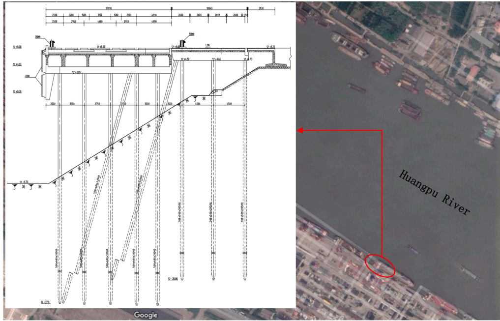
Fig. 2. Layout and cross-sectional diagram of the typical high-pile wharf in Shanghai Port.
