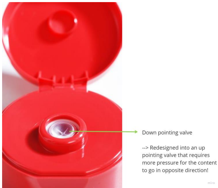
Figure 48: Explanation of integration ketchup valve
