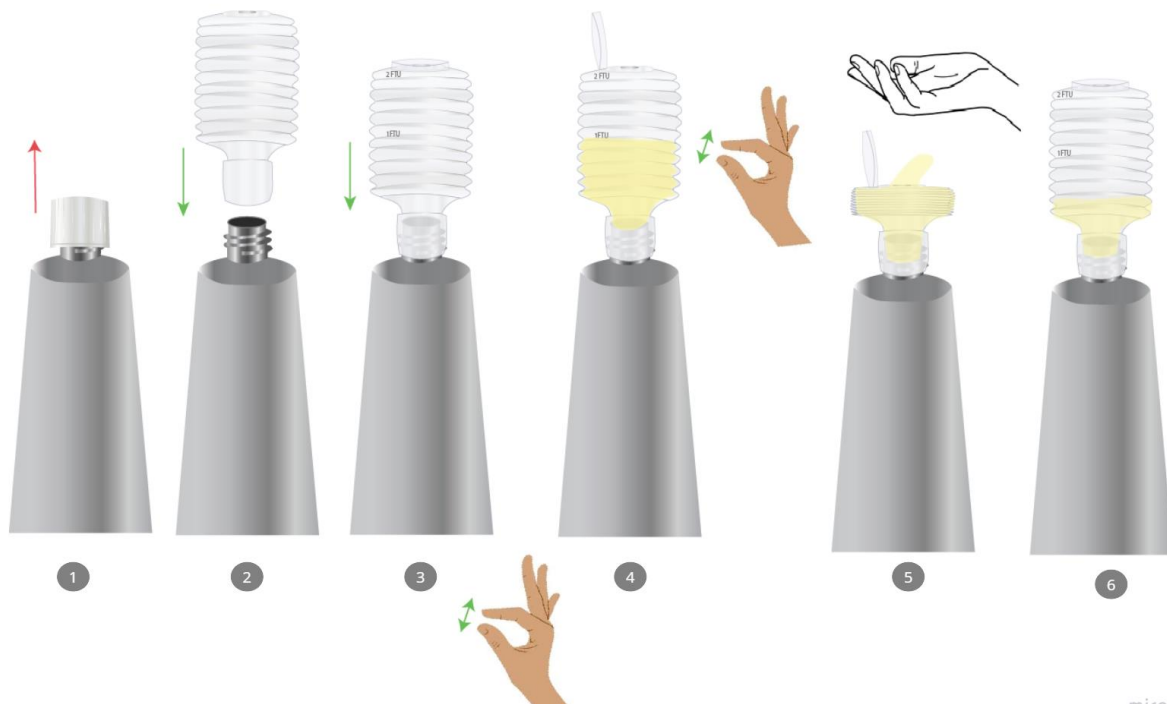
Figure 17: Dosing mechanism - Option 2
