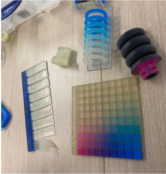
Figure 33: Examples PolyJet printed models
