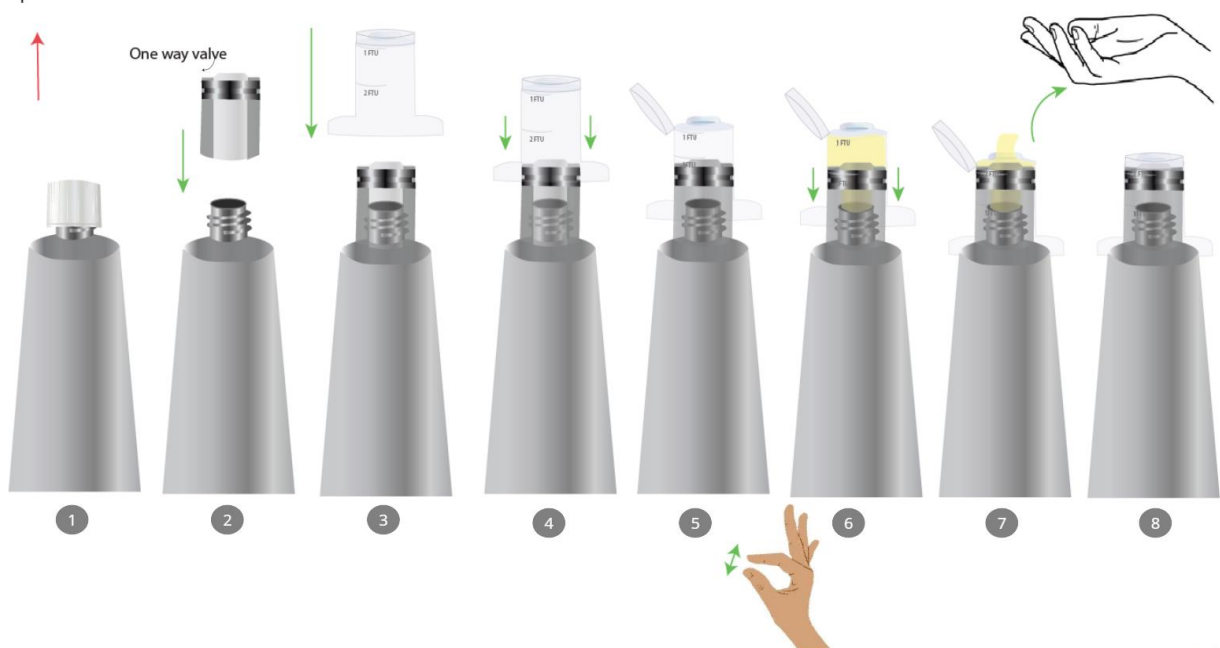
Figure 16: Dosing mechanism - Option 1, step by step working explanation.
