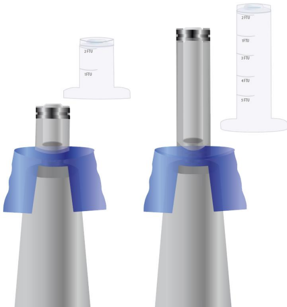
Figure 18: Adjustments in dosing mechanism
