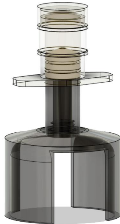
Figure 30: Plunger and barrel 3D model
