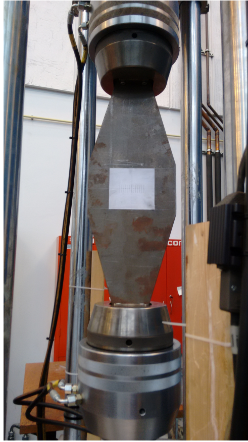
Figure 3.4: Test specimen clamped in the universal tensile testing machine
