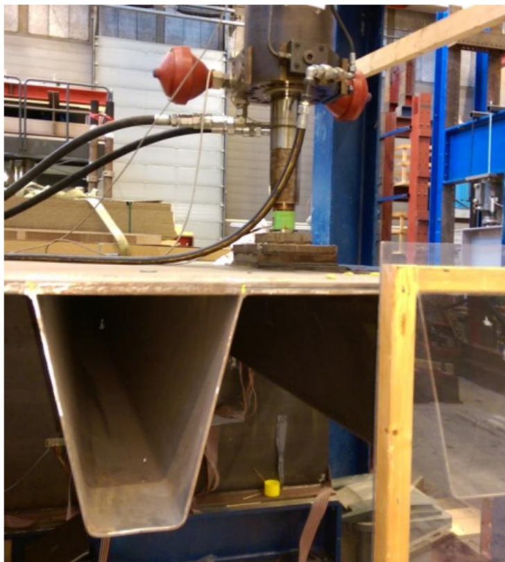
Figure 3.15: Loading on the bridge deck responsible for propagation of the fatigue crack
