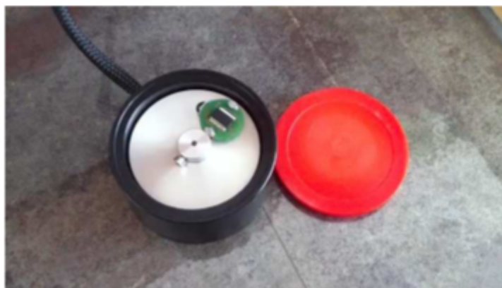
Figure A.1: Hall sensor inside the CrackGuard I
