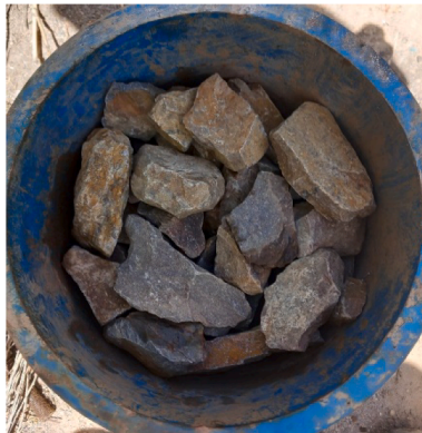
c Ballast specimen inside the main mold (0% CR)
