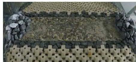
Figure 6.2: Crest-set up Grigoris with rear slope
