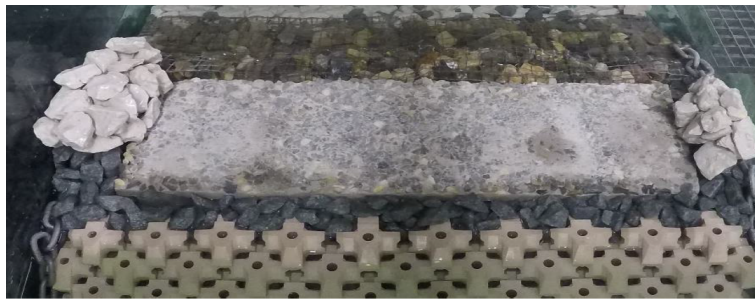
Figure 2.13: XblocPlus, rock fill and stiff element [13]
