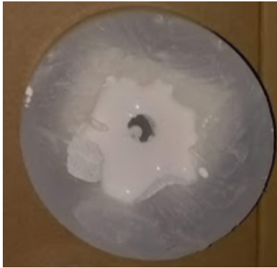
Figure D.4: Mould filled with Acrystal Aqua
