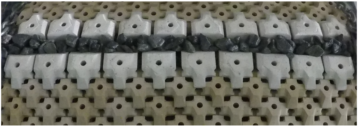
Figure 7.27: Crest armoured with 'Extended bottom blocks'
