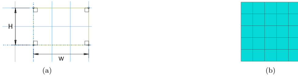
Figure 4.1: An overview of the geometry of the steel plate model (a), where H is the height and W is the width of the plate. A corresponding mesh (b) is constructed exclusively from quadrilateral plane stress elements
