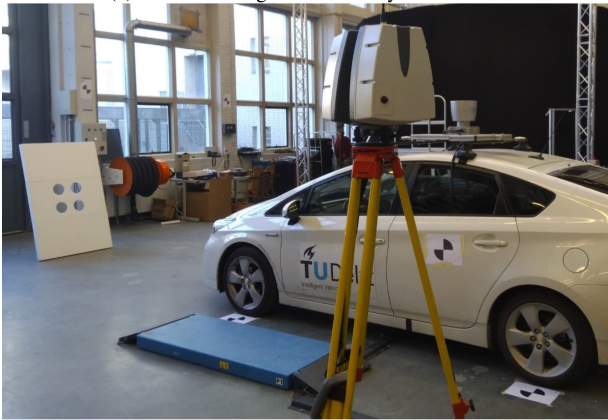
(b) Absolute calibration setup for a vehicle.
