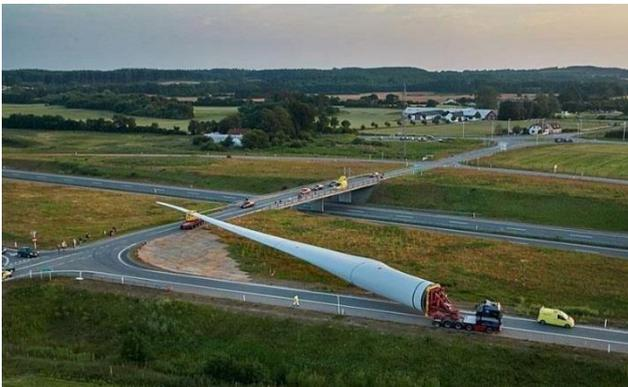
Figure 2.5 83.5 m long blade for Samsung S7.0-171 wind turbine [27].
