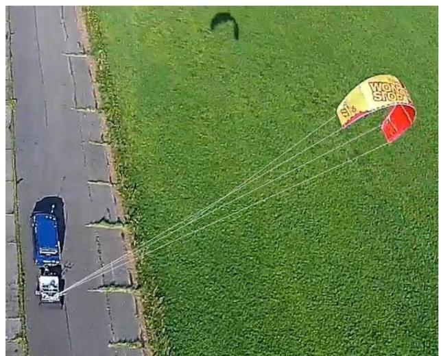
Figure 2.19 10 m<sup>2</sup> North Vegas kite towed by the TETA setup. Modified from [50].
