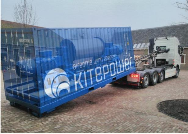
Figure 10.2 Kitepower system fitted into a freight container.
