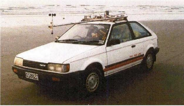
Figure 2.14 Car test rig designed by Alexander and Stevenson [44].
