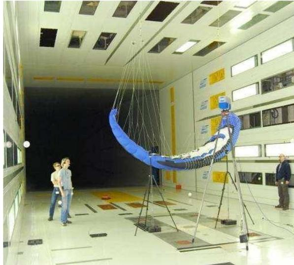
Figure 2.13 De Wachter analysing a 6 m<sup>2</sup> ram-air kite in the 8 x 6 m wind tunnel test section [42].
