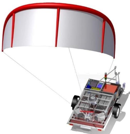
Figure 2.18 Schematic design of the towing test bench (TETA) developed by Hummel [49].
