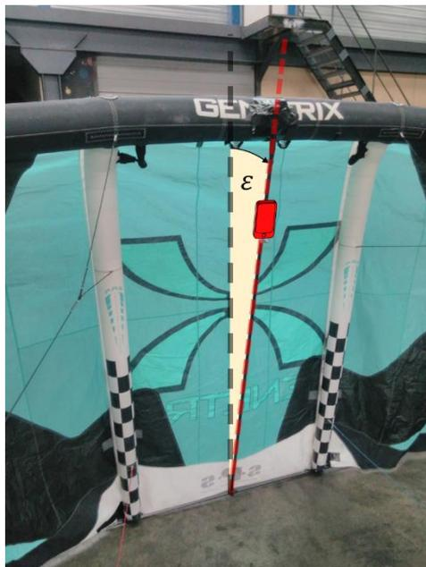
Figure 4.10 Angular sensor mounted on carbon rod.
