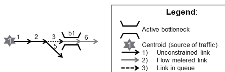
Figure 5.4: example where estimating demand matrices using method 1 and a single count on link 2 does not imply a positive effect on the fit on link 3
