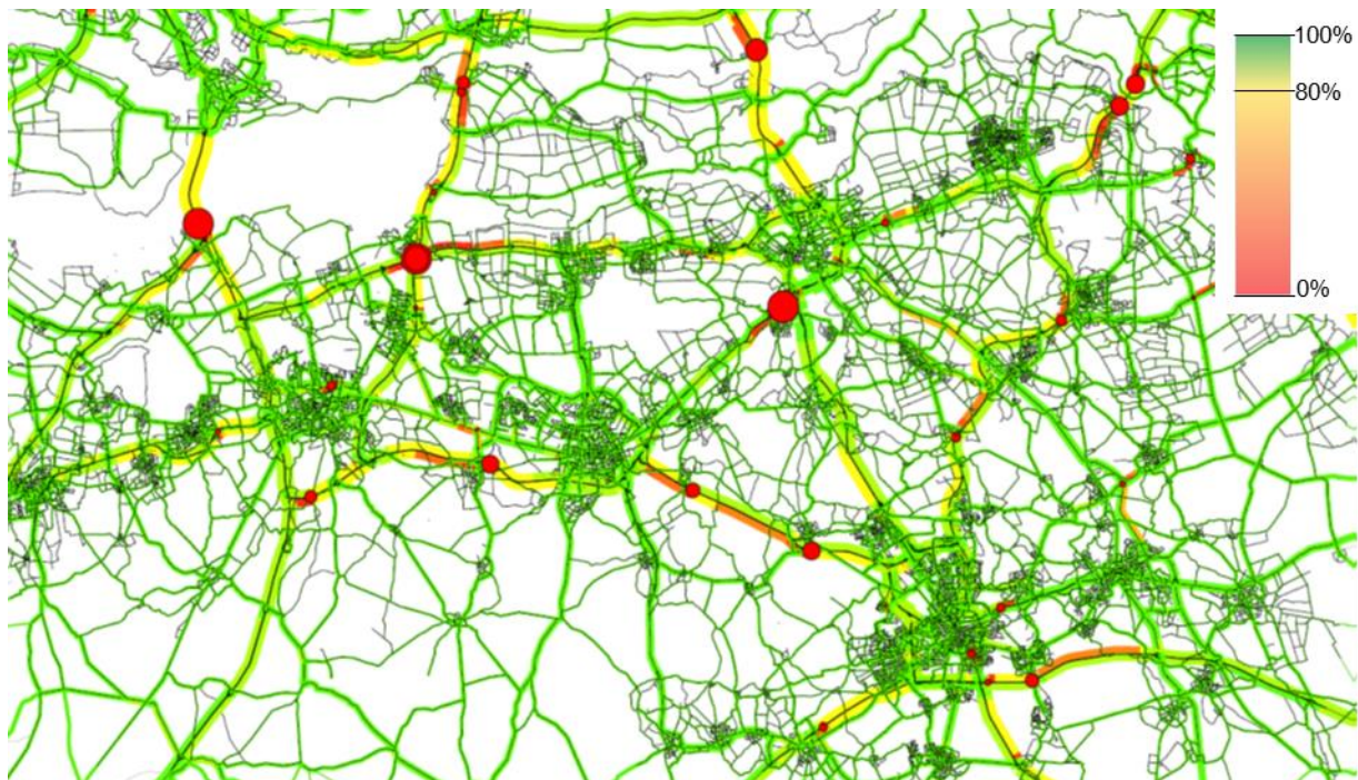
Figure 6.8: (study area of the) BBMB network: assignment results of prior OD matrix (width: flow; colour: speed as percentage of maximum speed; pie charts: number of vehicle hours spent in (vertical) queue)
