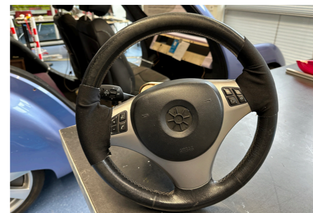
Figure 54: Steering wheel prototype with the covered vibration motors.
