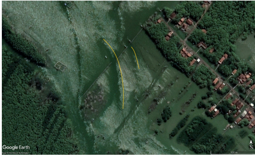
Figure 4.4: Streak lines of current patterns in the presence of permeable dams in Timbulsloko. Elevated flow velocities through the gaps between the structures can be ascertained from the darker lines accentuated by the yellow curves.
