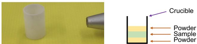
Figure 2.12: Picture of a TGDSC crucible with a pen tip for size reference (left) and a illustration of its contents after the sample and powder have been added (right)
