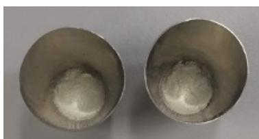
Figure 3.3: Picture of two platinum crucibles with  $\text{BaMo}_3\text{O}_{10}$  after the second cycle in the oven
