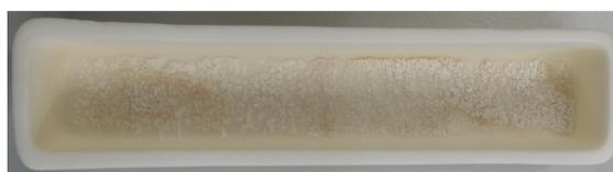
Figure 3.21: Picture of an aluminum oxide crucible with BaCs<sub>2</sub>(MoO<sub>4</sub>)<sub>2</sub> after the last cycle in the oven
