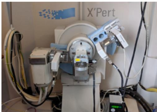
Figure 2.6: Philips PANalytical X'Pert PRO X-ray diffractometer [111]
