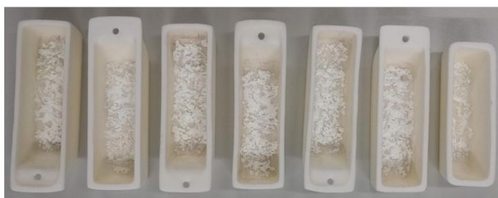
Figure 3.1: Picture of aluminum oxide crucibles with  $\text{BaMoO}_4$  after the last cycle in the oven
