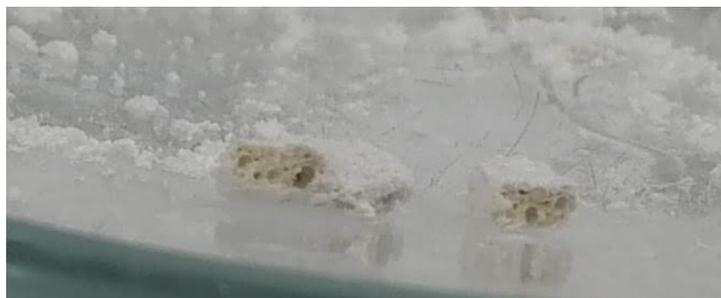
Figure 2.13: Picture of an agglomerated sample disk right after emptying a TGDSC crucible. The surrounding white powder is BN or  $\text{Al}_2\text{O}_3$ . The disk is ground into a powder so that it can be measured by XRD.
