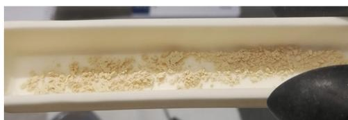
Figure 3.6: Picture of an aluminium oxide crucible with Ba<sub>2</sub>MoO<sub>5</sub> after the first cycle in the oven
