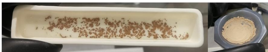
Figure A.6: Picture of aluminum oxide crucible with Ba<sub>2</sub>MoO<sub>5</sub> after the first cycle in the oven
