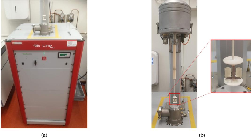
Figure 2.9: (a) Picture of the thermogravimetric differential scanning calorimeter that was used for measurements (b) The positioning of the reference crucible (left) and the sample crucible (right) suspended from the scale that is positioned on top of the TG/DTG machine
