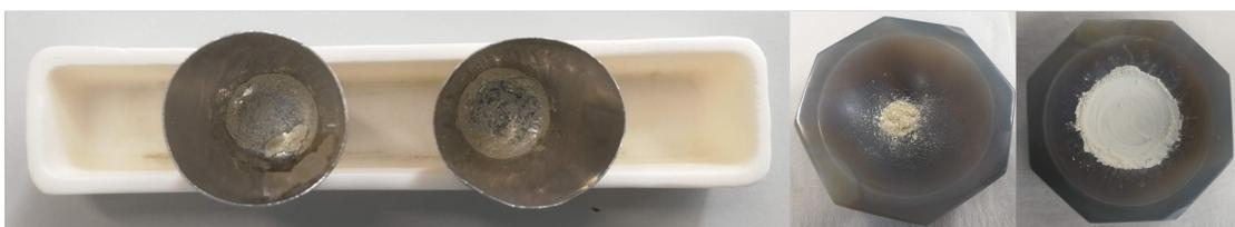
Figure A.4: Picture of two platinum crucibles with  $\text{BaMo}_3\text{O}_{10}$  batch FG13.3 after the third cycle in the oven
