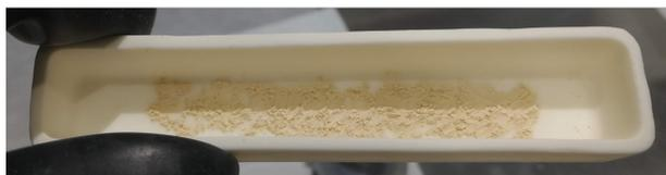
Figure 3.7: Picture of an aluminium oxide crucible with  $\text{Ba}_2\text{MoO}_5$  after the second cycle in the oven
