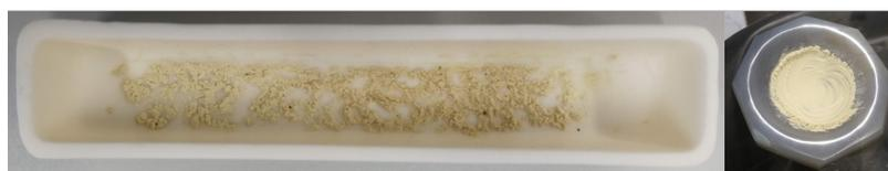
Figure 3.9: Picture of aluminium oxide crucible with Ba<sub>3</sub>MoO<sub>6</sub> after the first cycle in the oven
