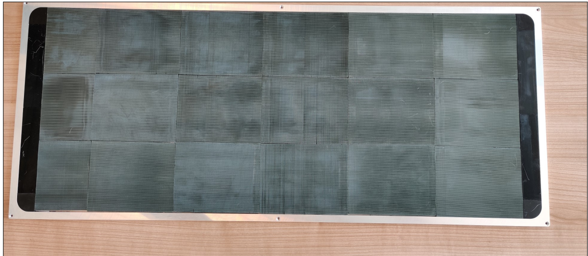
Figure 7.15: Wind tunnel test plate. Image taken before sealing minor unwanted cavities with tape.
