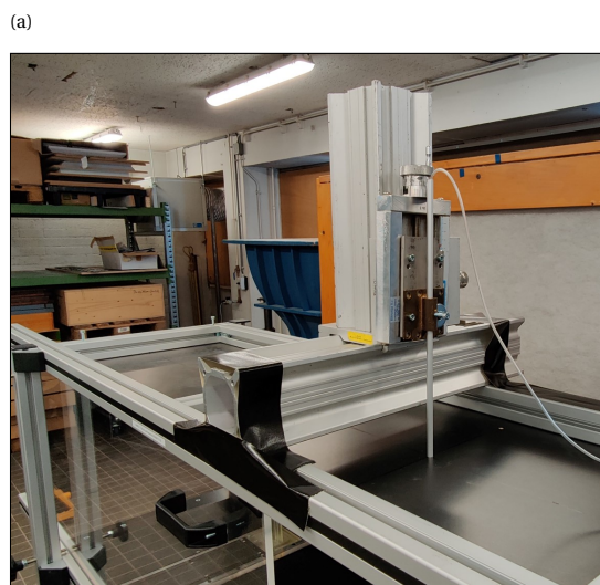
Figure F.1: Setup for pressure probe measurements. (a) Top view including traverse. (b) Side view, pressure probe and tubing above fibre test plate.
