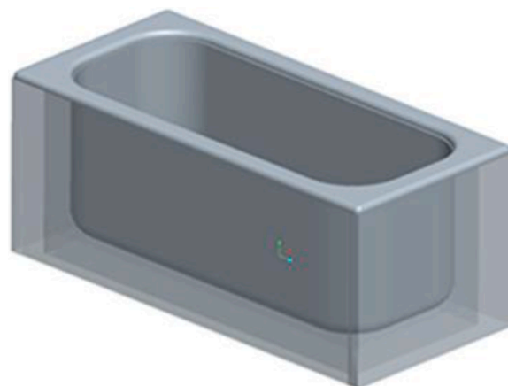
Fig. 30. PCM-based ice-cream container [101].
