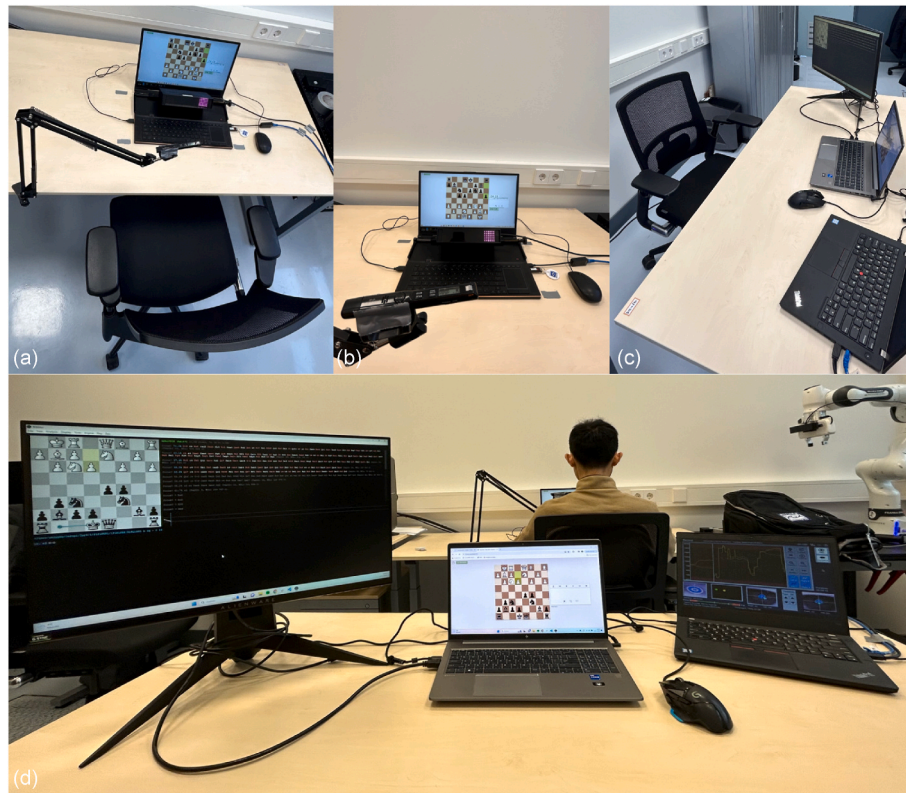
Fig. 1. (a) The seating position of the participant, with the voice recorder and the Portable Duo eye-tracker. (b) The participant's view during the experiment. (c) The seating position of the experimenter. (d) The view of the experimenter, containing from left to right 1) a monitor displaying the chess GUI (here for condition StockfishH), 2) a laptop where the experimenter plays chess against the participant, and 3) a laptop provided by SR Research, where the experimenter is able to check whether the Portable Duo is collecting eye-gaze data.
