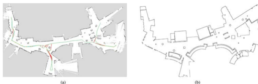
Figure 1: Maps of the first floor of MIT's Stata Center as presented in [8]. The left image shows the map created by the autonomously flying UAV developed in [8] using laser range finders. The right image shows the architectural floor plan.
