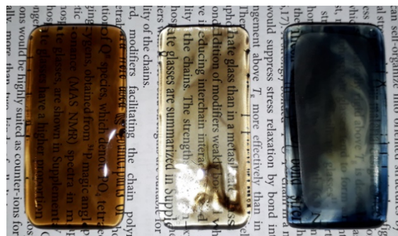
Fig. 6 Samples consisting of 15% slag, without the addition of B 2 O 3 , with the addition of 10% B 2 O 3 and 20% B 2 O 3 , respectively.
