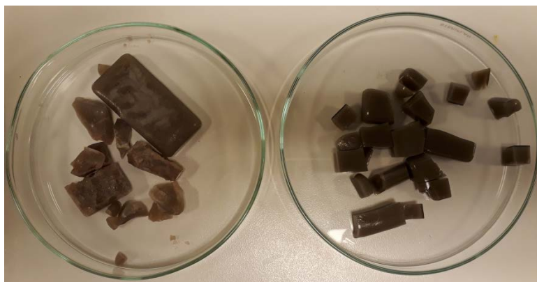
Fig. 3 Non-transparent samples containing 80KPO 3 -20Slag and 70KPO 3 -30Slag, respectively.
