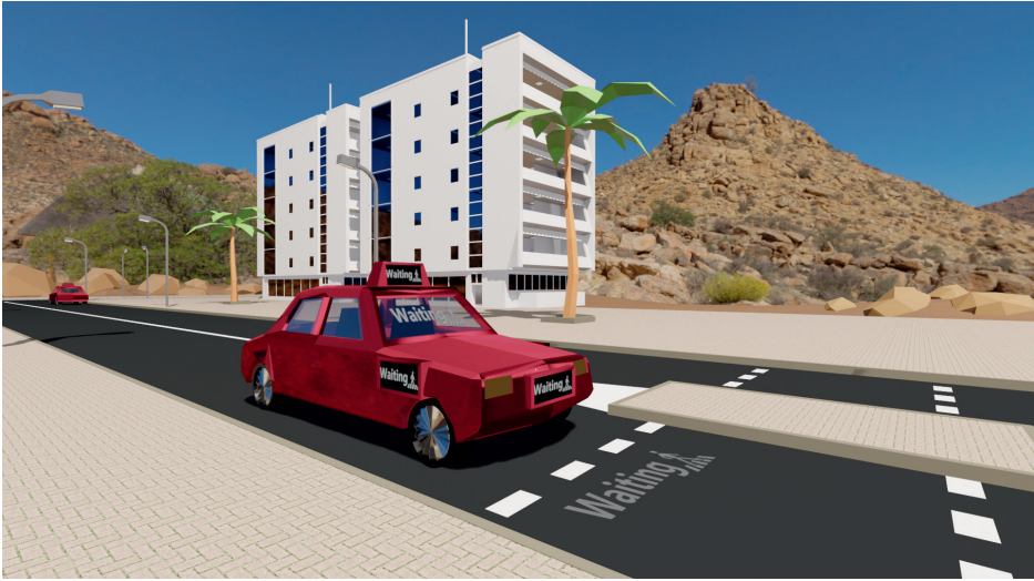
Figure 2. Car combining all five external human–machine interfaces (eHMIs). In the experiment, the car showed only one eHMI at a time. Here, the car has stopped for the pedestrian. The distance between the centre of the car and the camera (pedestrian) is 7 m longitudinal (i.e., parallel to the direction of the road) and 4.5 m lateral (i.e., perpendicular to the road). The white markings on the road were intended to create a pedestrian crossing on the road, without designated priority to the pedestrian.
