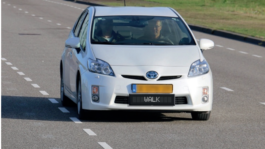
Figure 2. One of the six eHMIs used in the experiment. The person in the driver seat provided written consent for the publication of this photograph.
