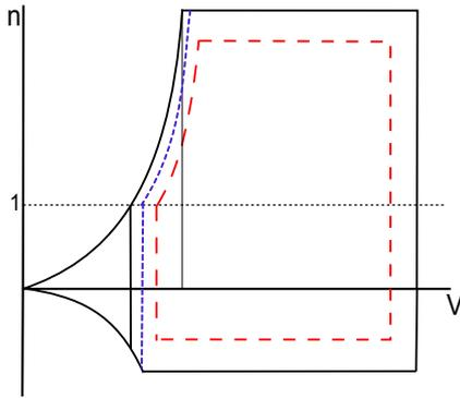
Fig. 1. Flight envelope with haptic feedback areas.
