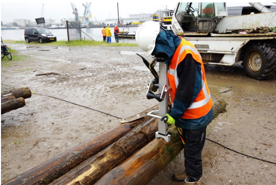
Figure 6: Microdrill in use on an excavated pile.
