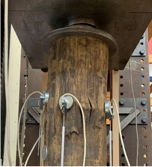
Figure 14: Failure in compression around knots
