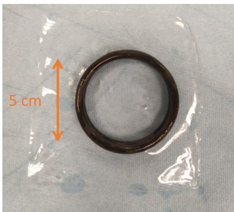
Figure 4.15: Cation exchange membrane at the end of the electrochemical reduction of CO 2 using Pb as cathode in a 0.7M TEACL in propylene carbonate solution at -2.5V vs Ag/AgCl. The anodic part of the reactor consisted of a Pt anode in 0.5M H 2 SO 4 . Both compartments were separated by an anionic exchange membrane. The membrane is swollen, which reduces the selectivity of the membrane.
