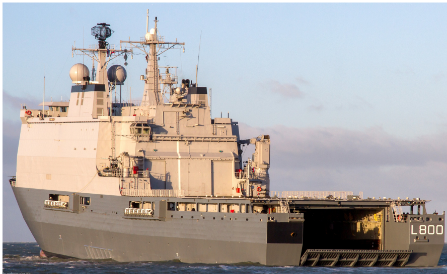
Figure 1.6: LPD opening the well-dock door and filling its ballast tanks [44]
