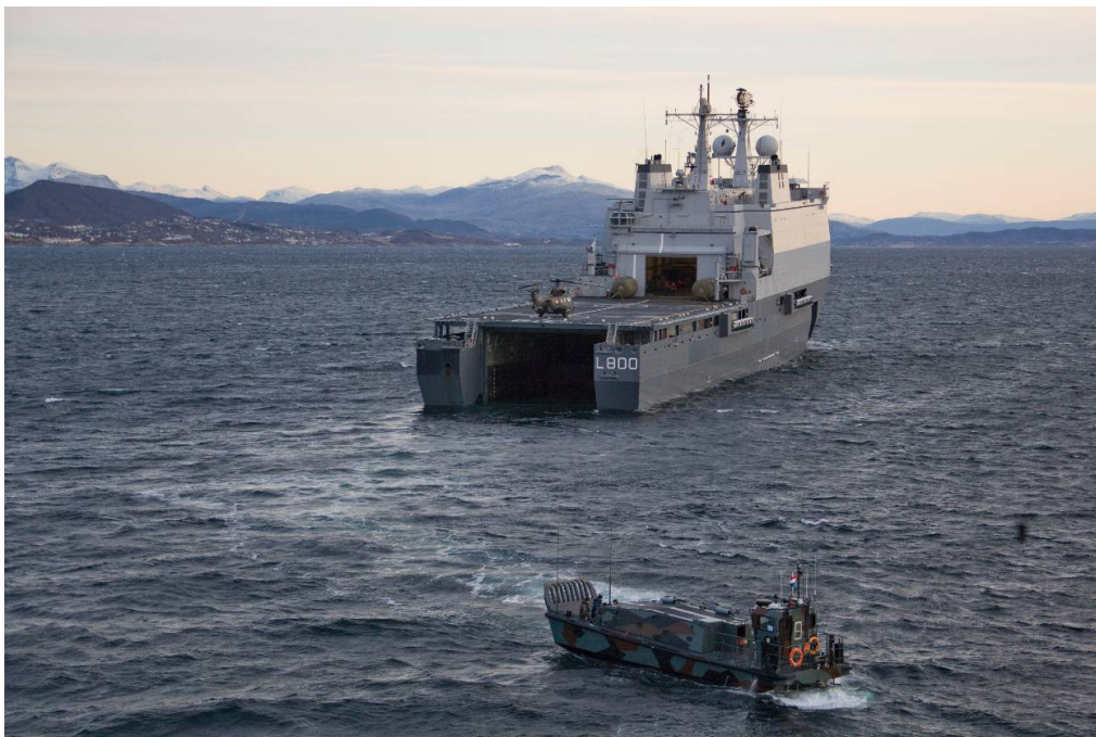
Figure 1.1: LPD with open well-dock and a landing vessel approaching at the stern [11]
