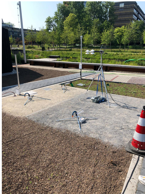
Figure B.7.: Radiometer setup for measuring albedos of various surfaces.
