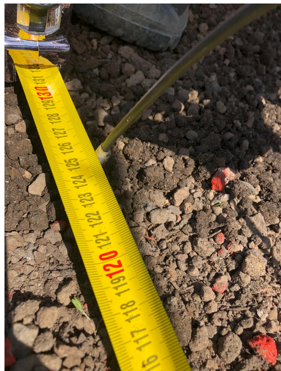
(b) Measurement of sensor location underneath roof substrate.
