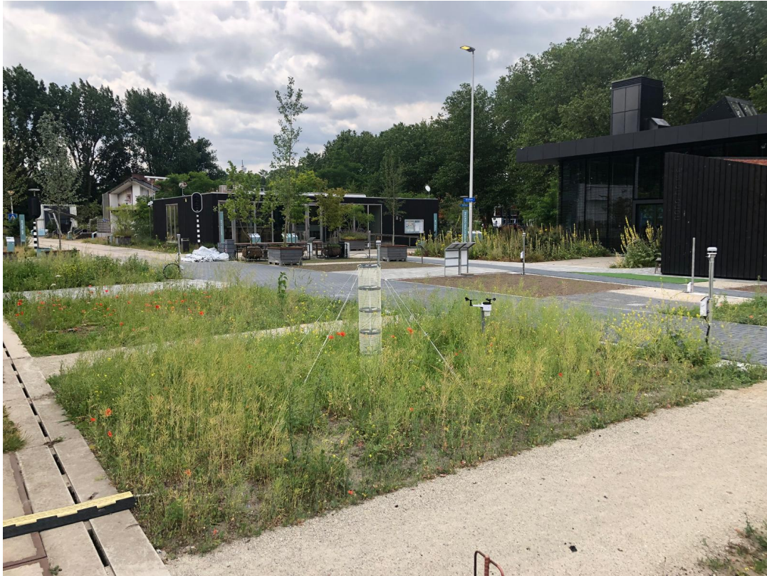
Figure B.8.: Measurement setup for measuring the vertical temperature profile above the surface, connected to the DTS system.
