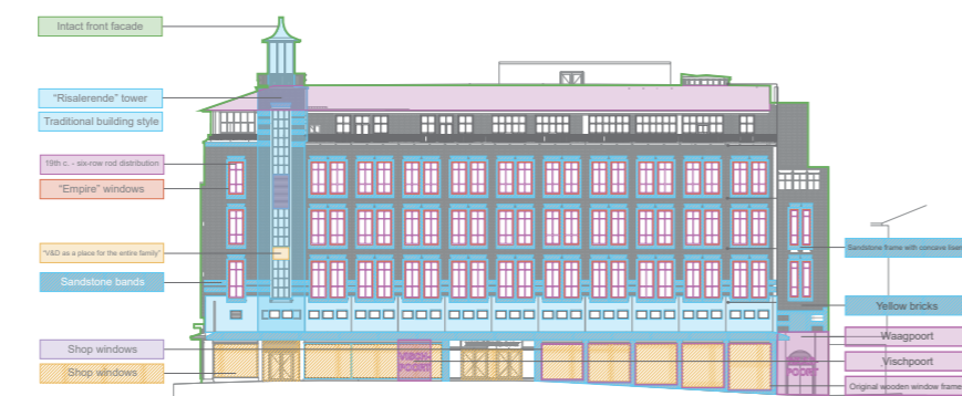
Figure 2 - Elevation of the facade of the Aalmarkt Visual analysis of the discovered layers and corresponding values and attributes
