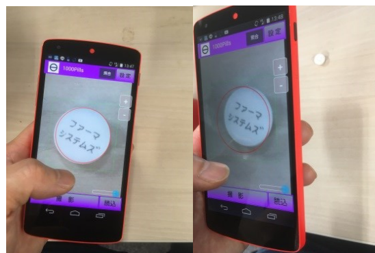
Fig. 5. Capturing query images using only a smartphone camera. Our simple GUI app helps non-expert users capture query images in an orthogonal view with suitable scaling and centering.
