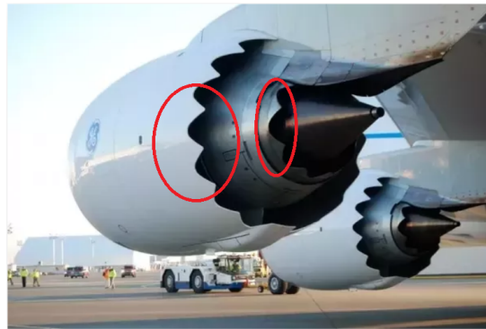
Figure 11.2: Chevrons on the Nacelle and Jet Exhausts
