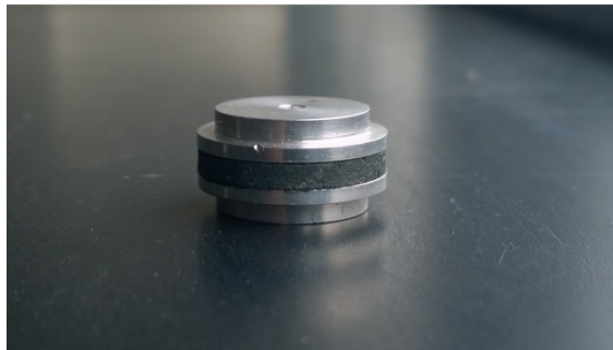
Figure 3.8 Parallel plates with the epoxy sample in between, after a dynamic viscosity measurement
