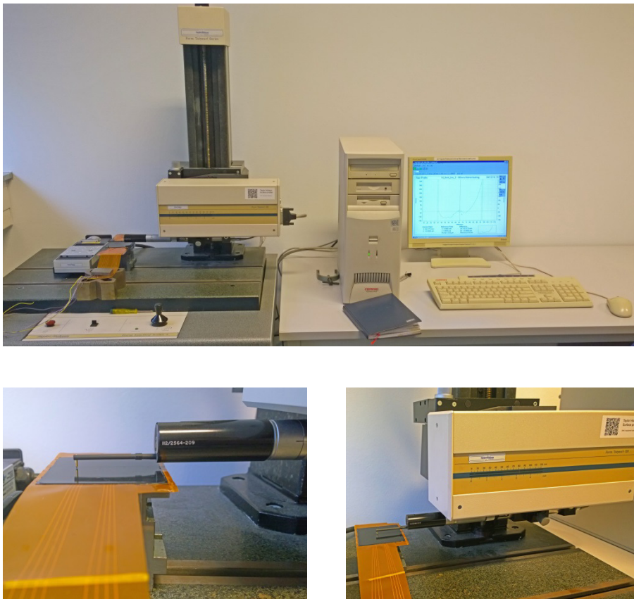
Fig 7.15 Warpage measurements conducted using the Taylor Hobson surface profiler “Form Talysurf-120”
