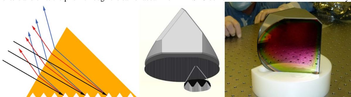
Fig. 1. The METIS Immersed Grating. Left: Immersed grating principle: light enters the prism through a polished entrance facet (black arrows); after diffraction at the grating facet the dispersed light leaves the prism through the entrance facet (red and blue arrows). Center: 3D drawing of the METIS IG, with the grating wafer detached from the prism. Right: The completed METIS IG demonstrator is ready to start the test campaign.
