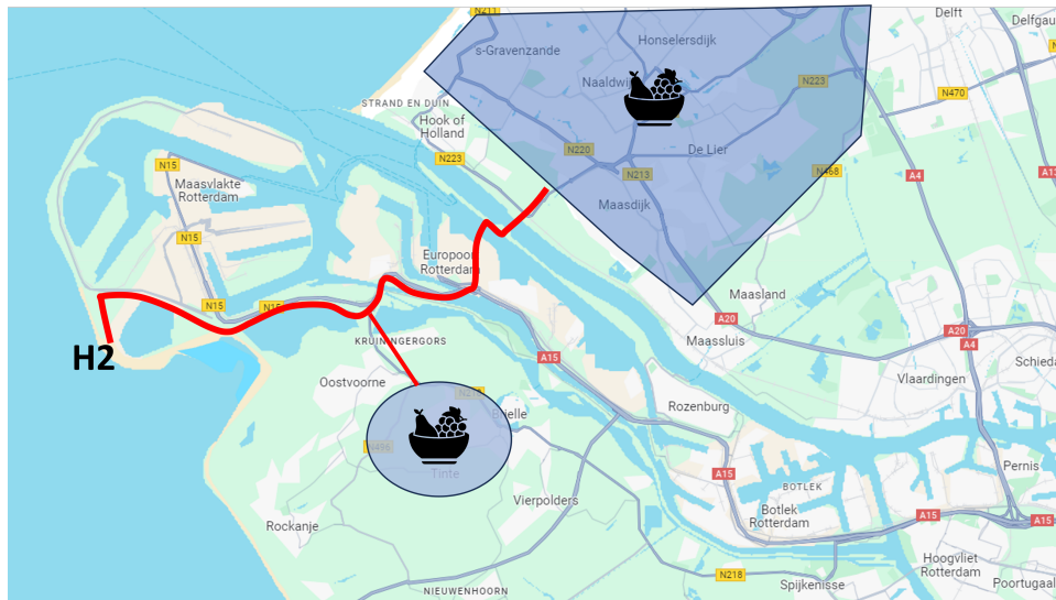
Figure 5.11: Schematic of greenhouse district heating case, red line represents 21.4 km of transport pipeline ( 25e+6 \text{ m}^2 of greenhouse area).
