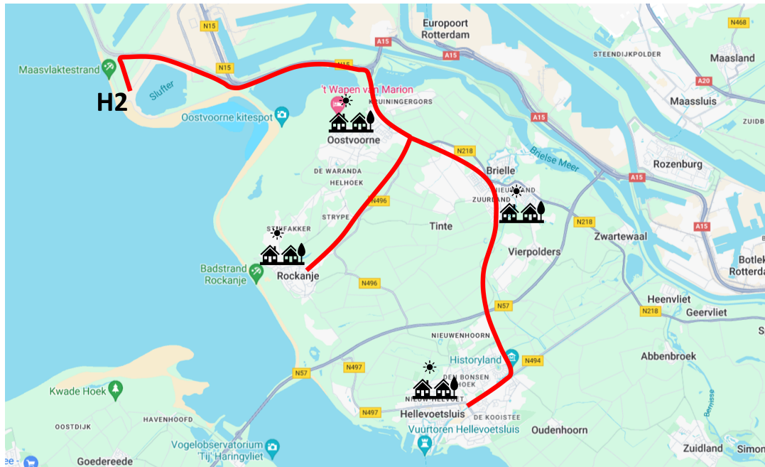
Figure 5.1: Schematic of urban district heating case, amount of pipeline: 27.4km. Amount of residential buildings: 28186
