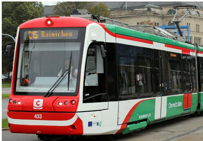
Figure 4-6: Citylink Chemnitz. The entry height difference between the white and red door is clearly visible. M.Bearton/Railwaymedia.
