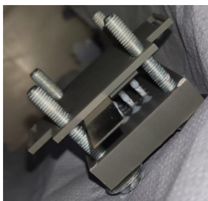
Figure 3.5 PTFE patterning test on a nickel plate. The plate extension shows the location of the electrode.
