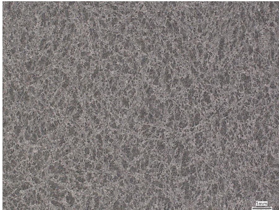
Figure A.1 OM image of a bare carbon electrode (x20)
