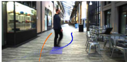
Figure 4.6: POV of the robot jointly predicting others and planning its own trajectory by learning from human expert demonstrations. Figure from [5]
