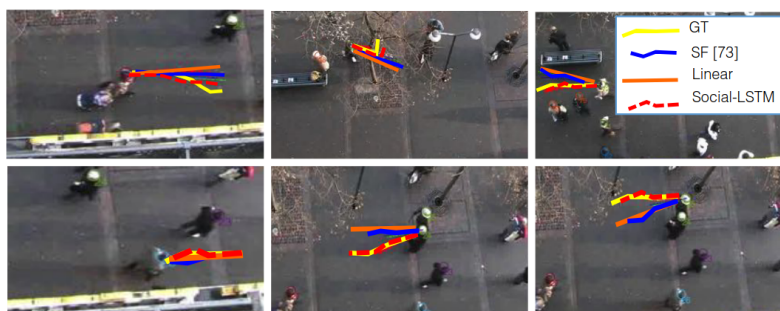
Figure 5.5: Figure from Social-LSTM publication comparing model outputs of CV, Social Forces and Social-LSTM [66]. The figure illustrates how the models can capture increasingly complex trajectory features respectively. Additionally note how the outputs are uni-modal.
