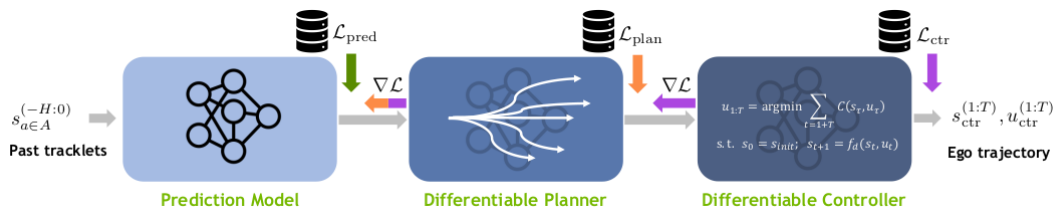
Figure 3.14: The authors of [17] present DiffStack a differentiable end to end modular architecture. By learning both a prediction model and planner parameters together, this leads to tight integration between both modules. This addresses problems often encountered when using learned prediction models with planners. In this manner the vehicle is capable of interactive behaviors while maintaining a sequential planning approach.
