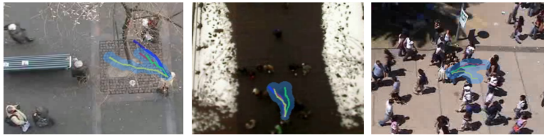
Figure 5.6: Figure from Social-VRNN publication [68], showcasing the multi-modal outputs of a variational approach. In this case a Variational Recurrent Neural Network (VRNN). The VRNN offers a variational approach to modelling time-series data, allowing for multi-modal outputs.
