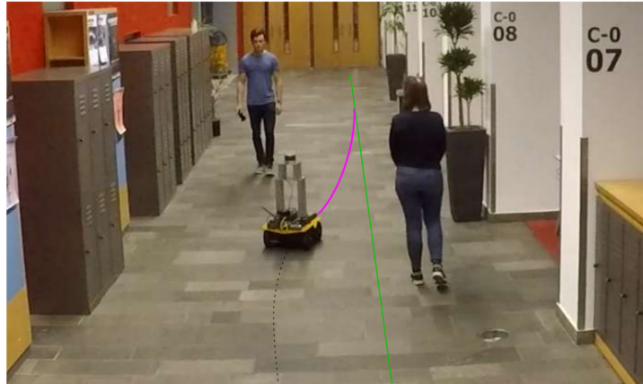
Figure 2.2: Illustration of MPCC reference tracking methodology. The green line represents the reference trajectory. In order to avoid a pedestrian it deviated from the reference but returns as soon as the pedestrian has been overtaken. This behavior is illustrated by the purple line representing the planned trajectory.
