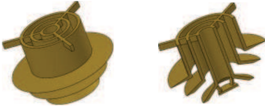
Fig. 2 Flow distributor/guide vanes, where it is possible to see the tripartite guide vane construction. It is mounted in the sudden expansion.
