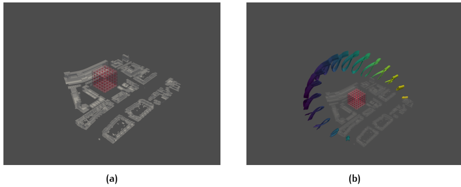
Figure 3.2: (a) The result of the first toy problem: In red a simple 5 \times 5 \times 5 'rubik's cube' with voxels of size 15m^3 and in light gray the imported environment. (b) The result of the sun pathing toy problem: the arrows are directed towards the centre of the lattice.
