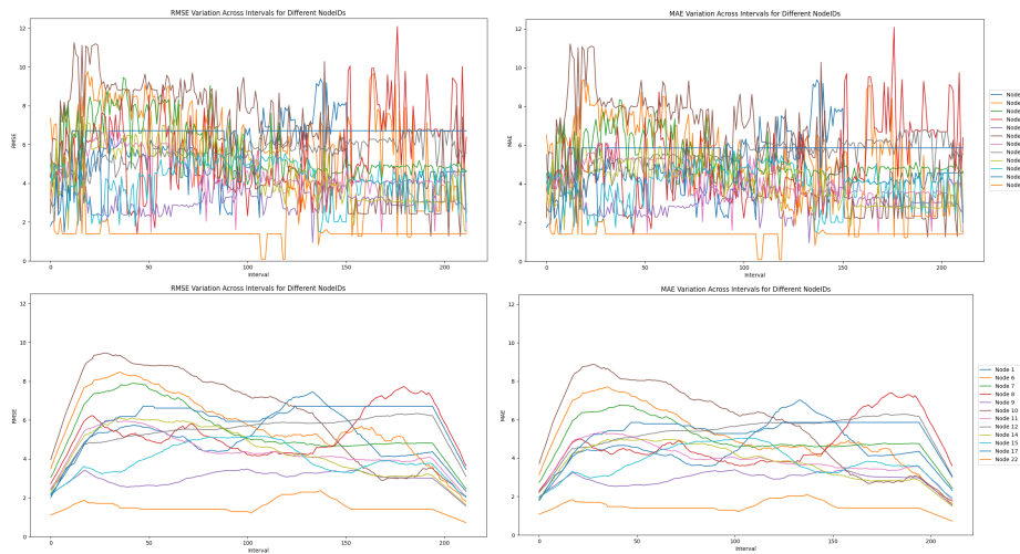
Figure I.1: Comparison of RMSE and MAE variations across intervals for different Node IDs, illustrating both the original and smoothed versions filtered with a 35-interval window. The top row depicts the normal data, while the bottom shows the smoothed versions.
