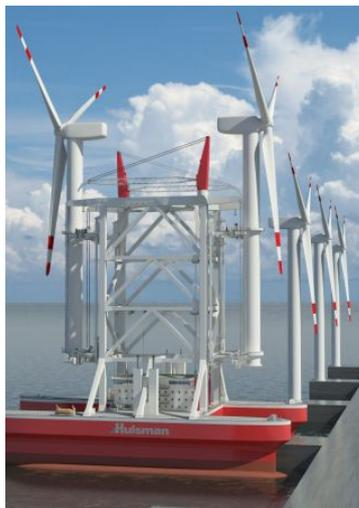
(b) Shuttle with two turbines
