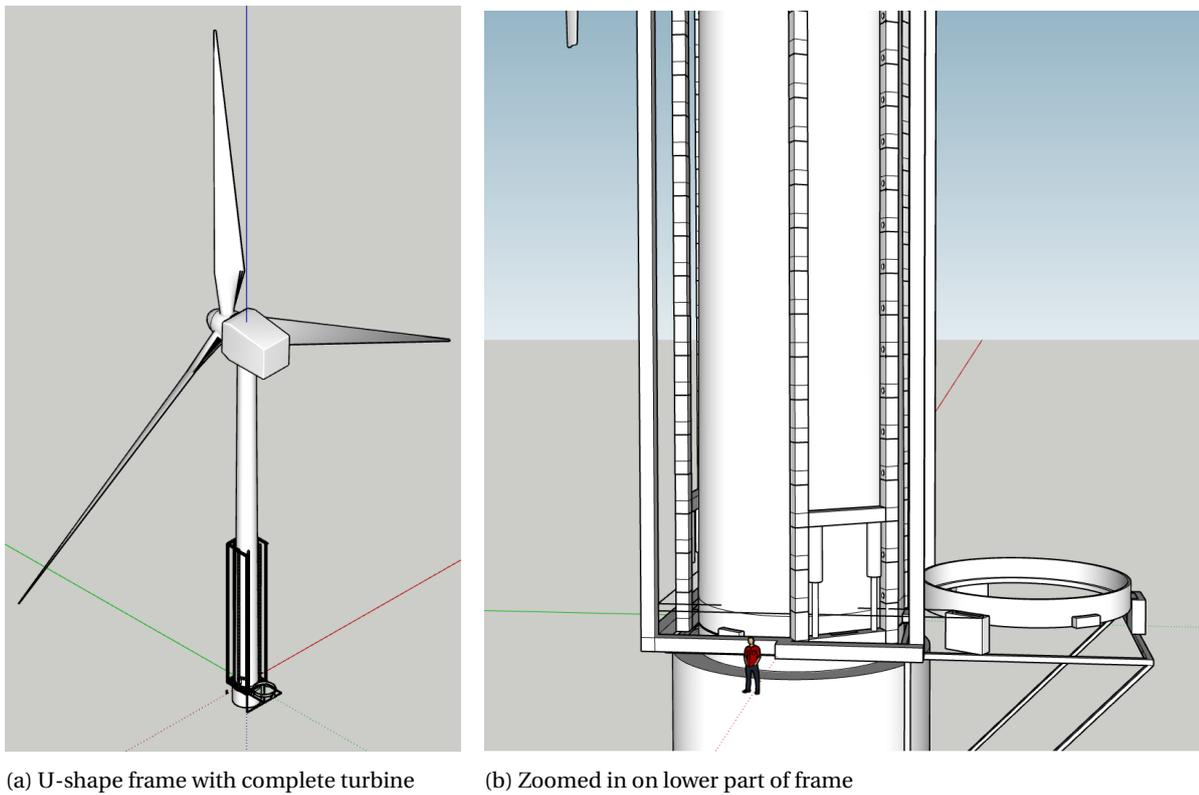
Figure 6.4: 3D impression of the U-shape frame
