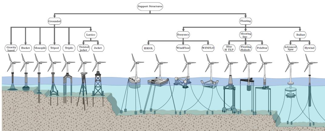
Figure 2.2: Types of support structures for OWTs (Rodrigues et al., 2016, p.14)
