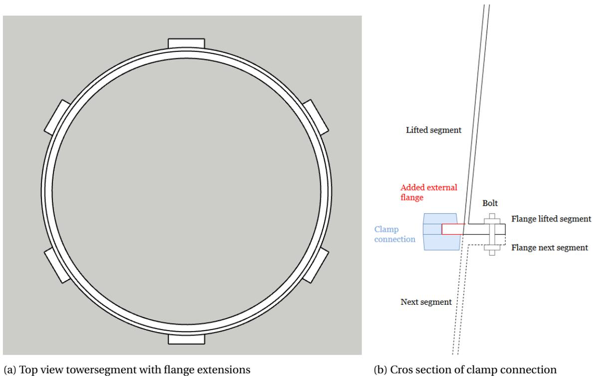
Figure 6.1: Illustrations of interface between tower segment and lift mechanism
