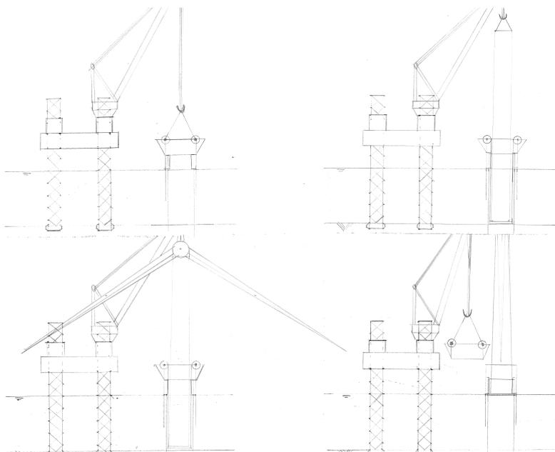
Figure 4.4: Drawings of lifting the turbine out of the monopile
