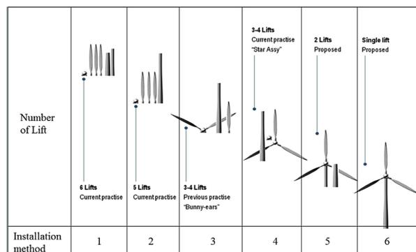
Figure 2.13: Different installation sequences (Ahn et al., 2017, p. 48)
