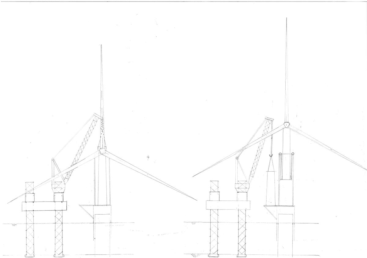
Figure 4.6: Visualisation of installation steps of bringing up tower
