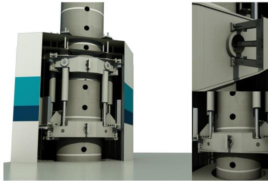
Figure 6.2: Jacking system, courtesy of GustoMSC
