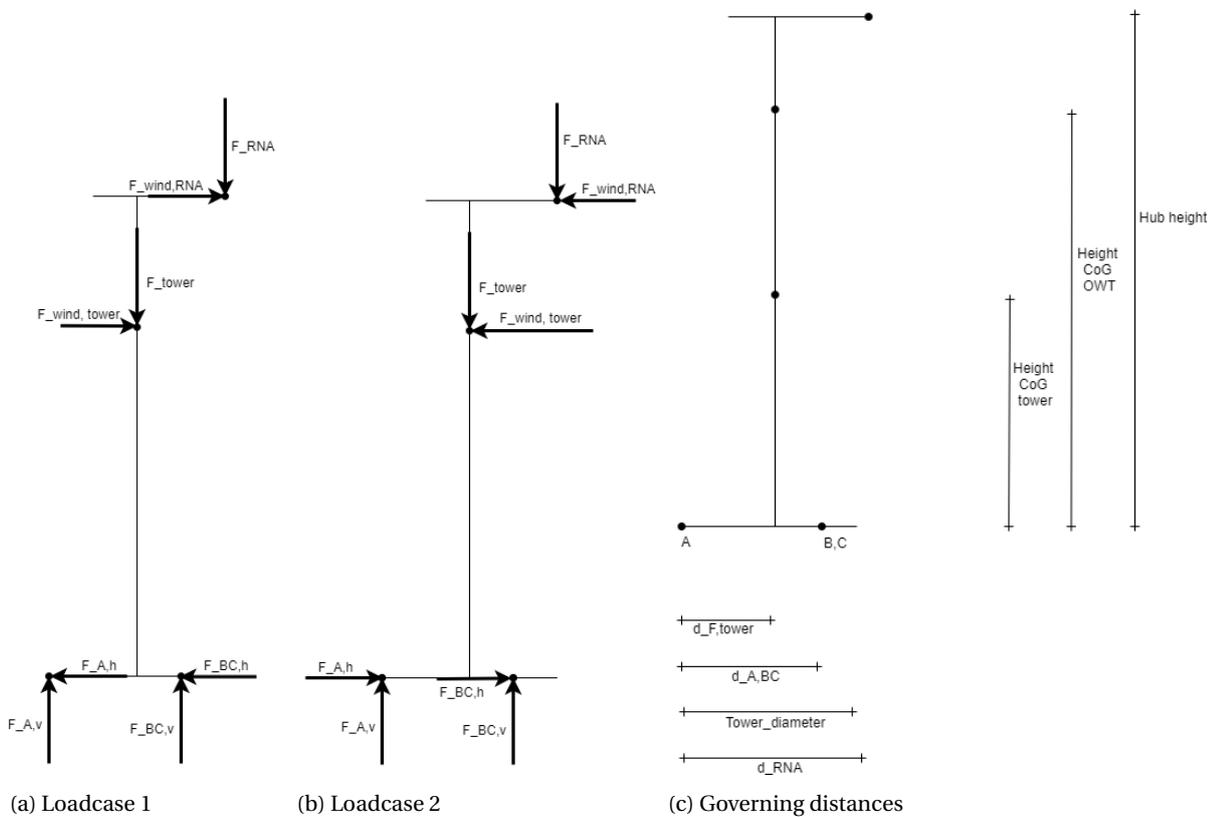
Figure D.6: Free body diagrams of governing load cases
