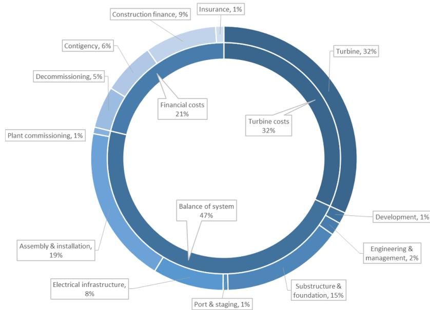
Figure 2.9: Capital expenditure breakdown of an offshore wind turbine. Data from (Moné et al., 2017, p.10)
