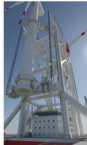
(c) Clamping mechanism on shuttle
