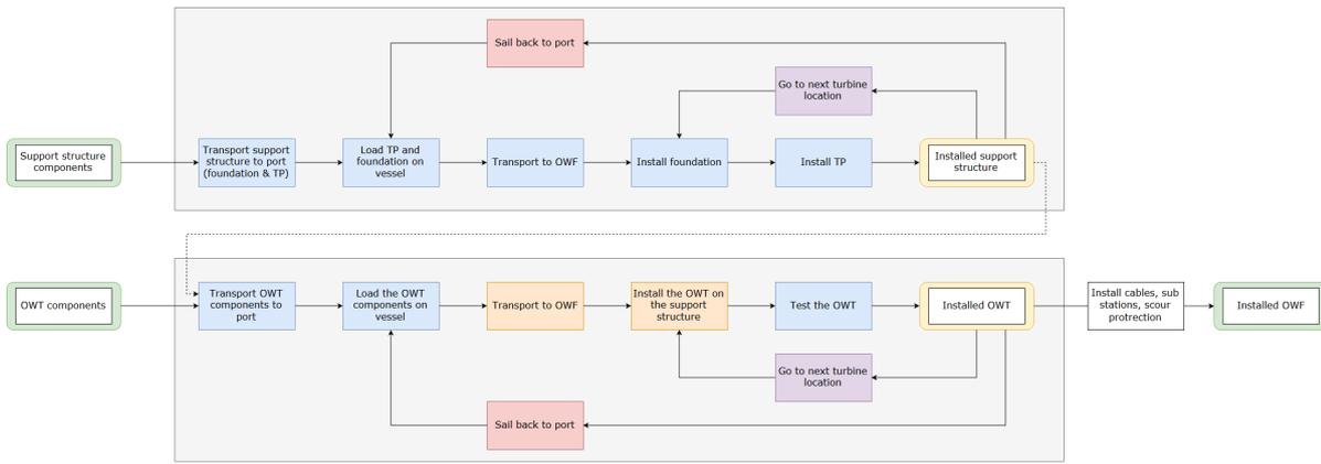
Figure 2.12: Flowchart of T&I of an offshore wind farm
