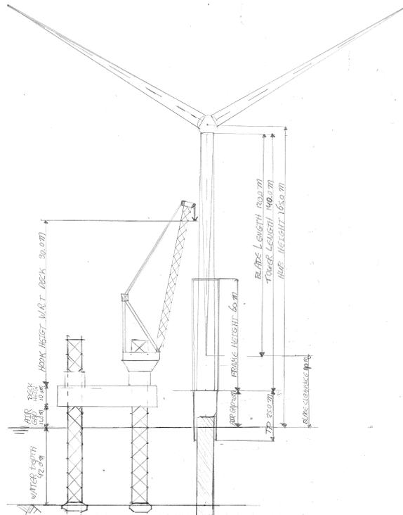
Figure 5.2: Jack-up system with height indication
