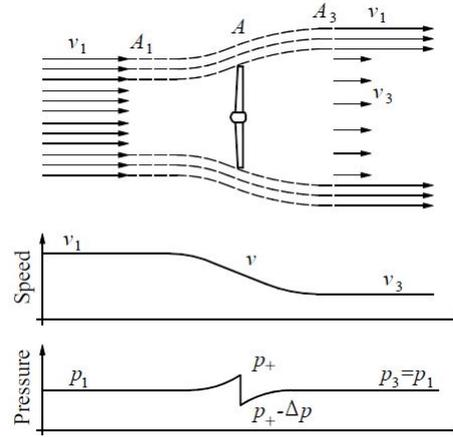
Figure D.1: Stream tube around a rotor, change in wind speed and pressure difference (Gundtoft, 2009, p.3).
