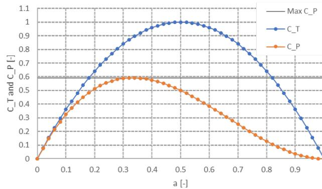
Figure D.2: Thrust and power coefficient as function of the induction coefficient
