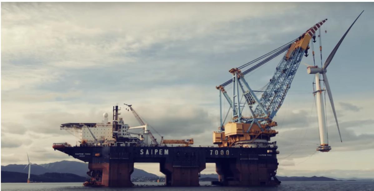
Figure 2.16: Saipem 7000 transporting a wind turbine (Offshorewind, 2017)
