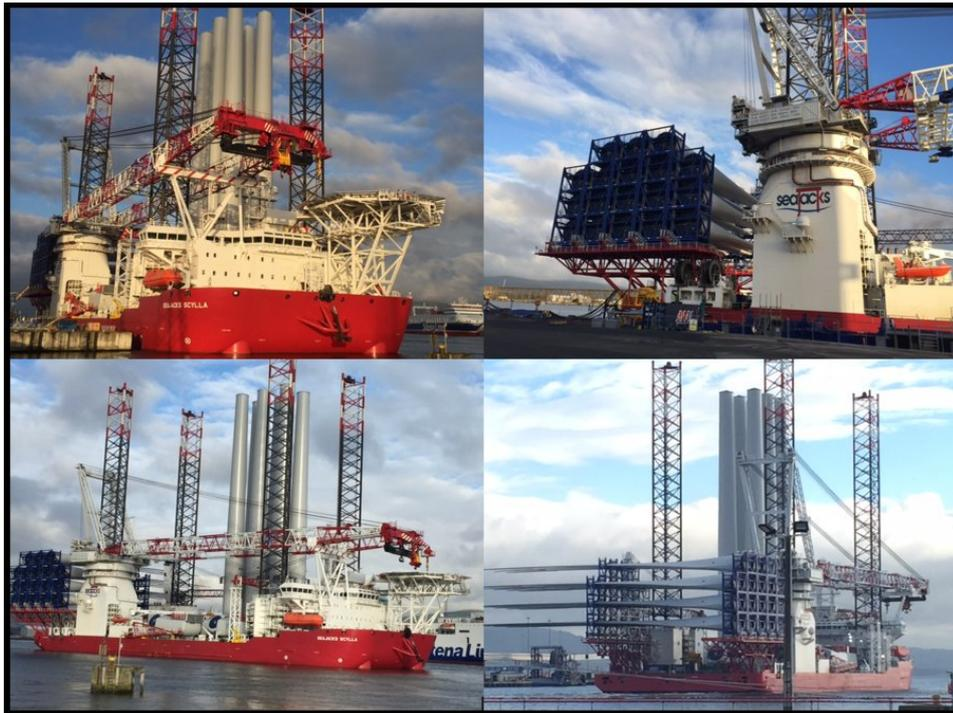
Figure 2.14: Jack-up vessel Seajacks Scylla. Courtesy of Seajacks
