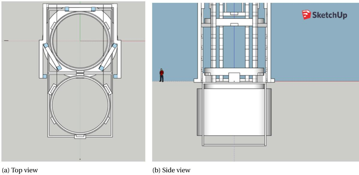
Figure 6.3: U-shape frame. The tower segments are not displayed completely so the different components of the lift frame are still visible
