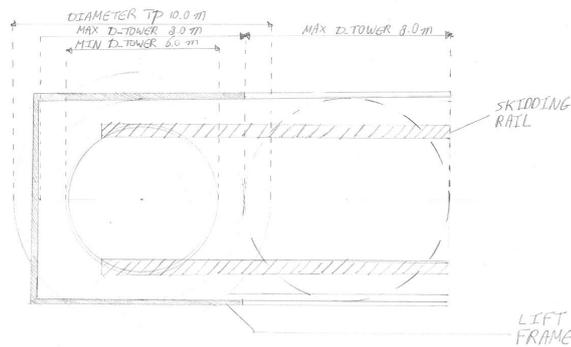
Figure 5.3: Top view of total frame, with lift frame left and skid part right
