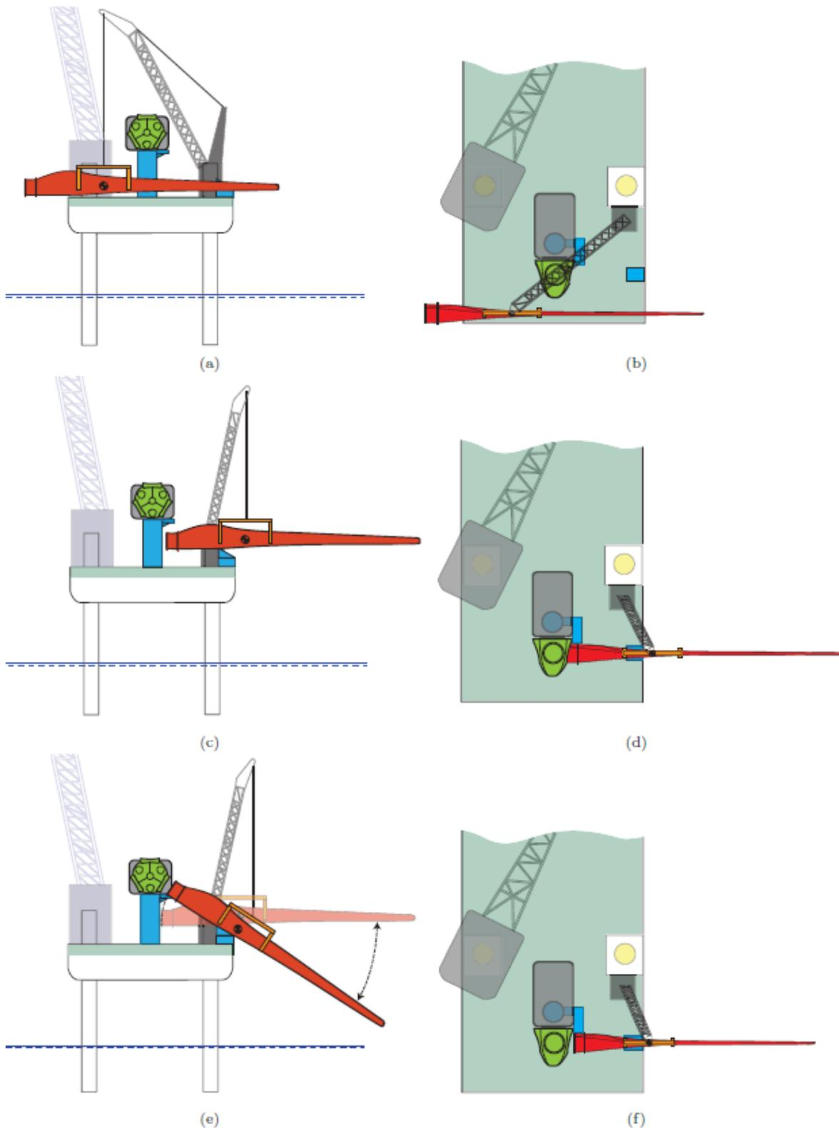
Figure 5.4: Assembly tower of (Strien, 2011, p.141). Steps of manipulation of the blade towards the pre-assembly of hub and nacelle by use of blade handling tools. [left] Front view [right] Top view. (a,b) Pick up from stack position. (c,d) Move to the starboard of the vessel. (e,f) Tilt to the desired angle of 30 degrees by using the guidance frame
