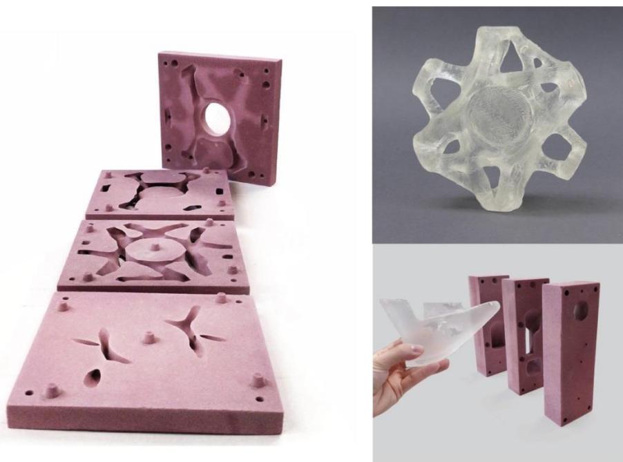
Fig. 11 3D-printed sand moulds produced by ExOne and the resulting cast glass components for a topologically optimized cast glass grid-shell node by (Damen 2019) (left and top right) and for a structurally optimized cast glass column by (Bhatia 2019) (bottom right).
