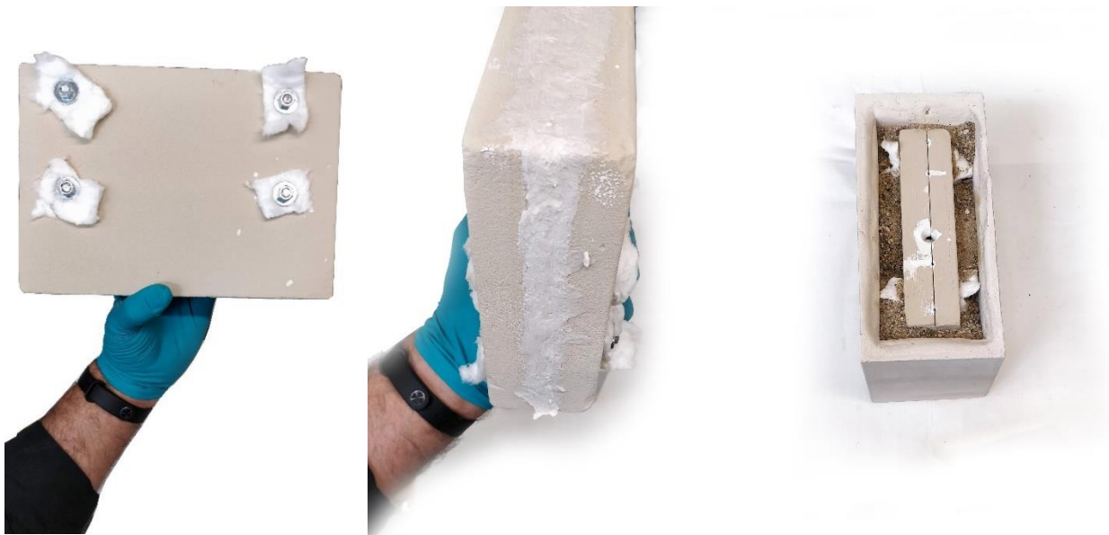
Fig. 9 Safety measures employed at the 3D-printed sand moulds prior to casting (Geometry 1).
