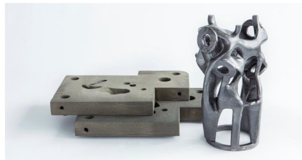
Fig. 6b) Cast steel node made in 3D-printed sand mould by Arup. Source: Arup/Davidfotografie.
