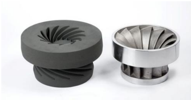
Fig. 6a) Example of metal casting (right) by a 3D-printed sand mould (left). Derived from www.voxeljet.com .
