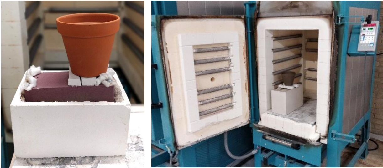
Fig. 10 Experimental set-up of the mould inside the kiln (left: Geometry 2, right: Geometry 3).
