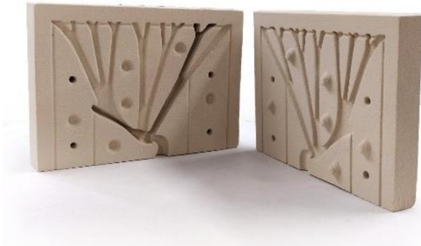
Fig. 8a) 3D-printed mould using Anorganic binder of Geometry 1.
