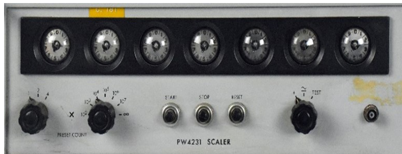
Figure 9. Philips Scaler 4231 using this special ZM 550 tube
